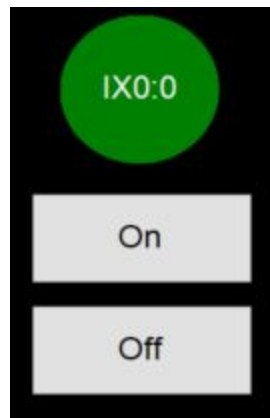
Figure 1: Reading Digital Inputs & Outputs with LED Indicators. Writing Digital Outputs with push buttons
