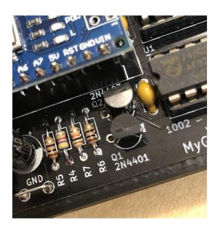
The silkscreen print for Q1 and Q2 has been fixed in PCB versions 1.8b onwards.
