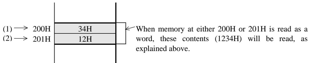
Word boundaries do not exist in program memory space. They also do not exist in program memory space accessed through the ROM window (table segment). This operational difference between data memory space and program memory space arises due to differences in address generation hardware.
