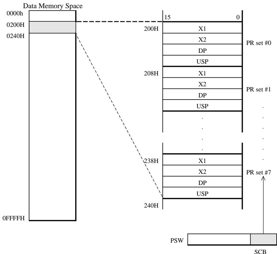
The pointing register set to be used is selected by the SCB field in the PSW. The following table shows the relation between SCB field values and the pointing register set selected. Immediately after reset, pointing register set #0 will be selected. The initial values of all pointing registers are undefined.
