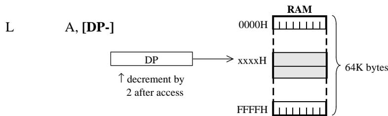
If an odd address is specified, then the data word starting at the even address immediately below it will be accessed (→word boundary).
