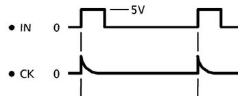
The capacitor coupling allows reset pulses to be supplied intermittently from the  $\overline{\text{RESET}}$  pin whether the input level (IN) is high or low.
