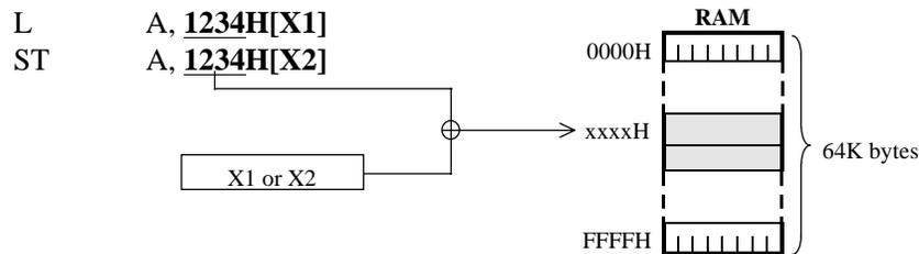
If an odd address is specified, then the data word starting at the even address immediately below it will be accessed (→word boundary).
