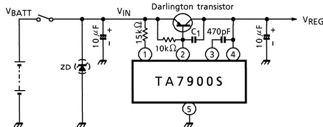
\* Select a  $C_1$  value according to the working condition -- typically above 2000pF.
