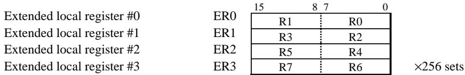
The local register sets are allocated in the 2048 bytes starting from address 200H in the fixed page of data memory space. They are allocated in order #0, #1,..., #255 from low address to high. Within each local register set, R0 to R7 are allocated to memory in that order from low address to high.
