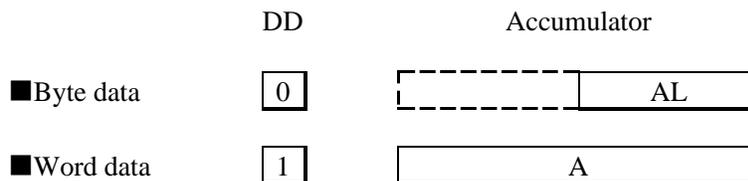
The type of calculations that use the accumulator (A) is determined by DD. Instructions that affect this flag are accumulator load instructions, clear instructions, and type conversion instructions, as well as instructions that directly set and reset the flag. Instructions affected by this flag are basically those that leave calculation results in A and those that store the contents of A.
