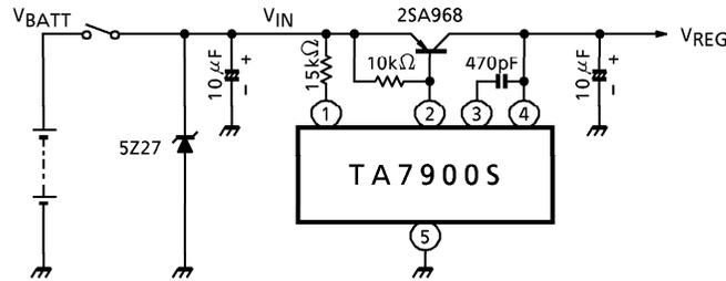
EXAMPLE OF APPLICATION CIRCUIT USING DARLINGTON TRANSISTOR
