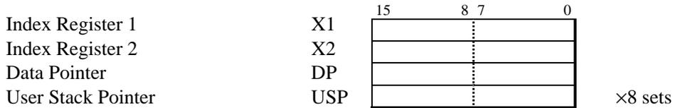
The pointing register sets are allocated in the 64 bytes starting from address 200H in the fixed page of data memory space. They are allocated in order #0, #1, ..., #7 from low address to high. Within each pointing register set, X1, X2, DP, and USP are allocated to memory in that order from low address to high.
