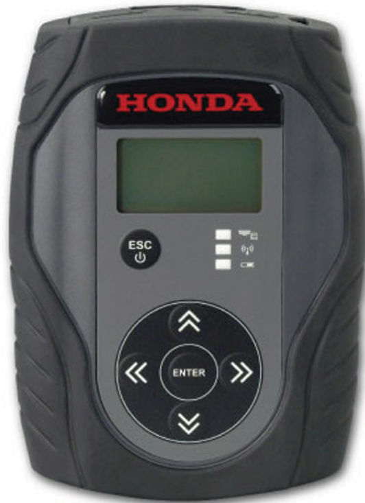
Figure 8. Honda / Acura Modular Vehicle Communications Interface (MVCI). [7]
