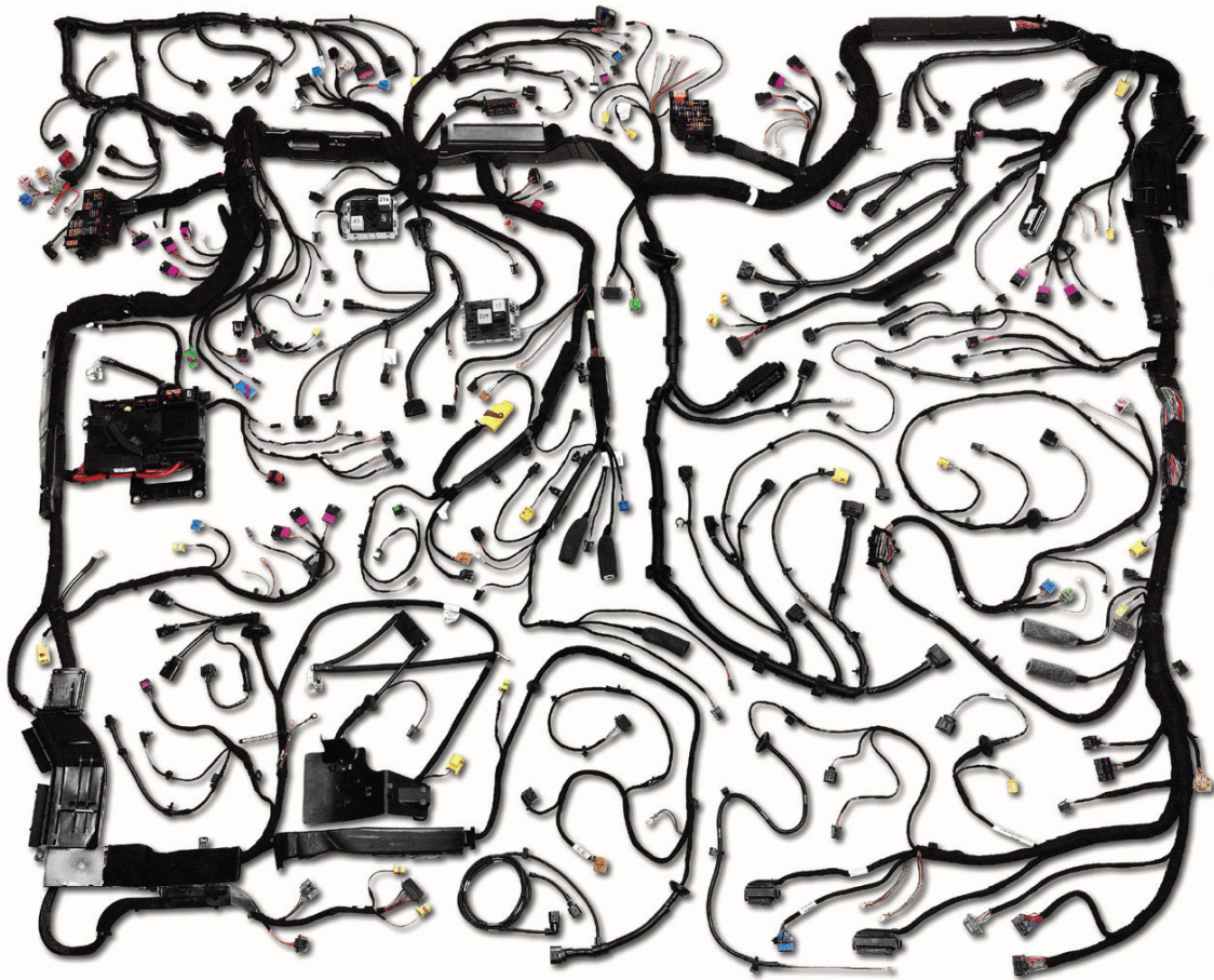
Figure 5. A Typical Wiring Harness In A Passenger Vehicle [4]
