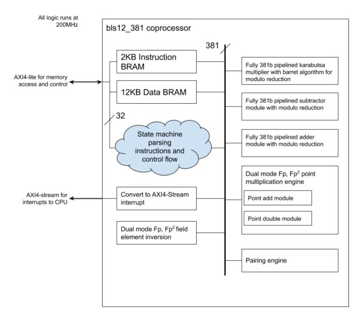
The coprocessor operates on a shared 381 bit bus with a main state machine with pointers into a data and instruction memory (implemented using Xilinx Ultra RAM on the FPGA). The top level multiplier, adder, and subtractor are all fully pipelined (so a new result each clock) and are resource shared with the entire coprocessor (so inversion block, dual mode point multiplier, pairing engine,... all use this).
