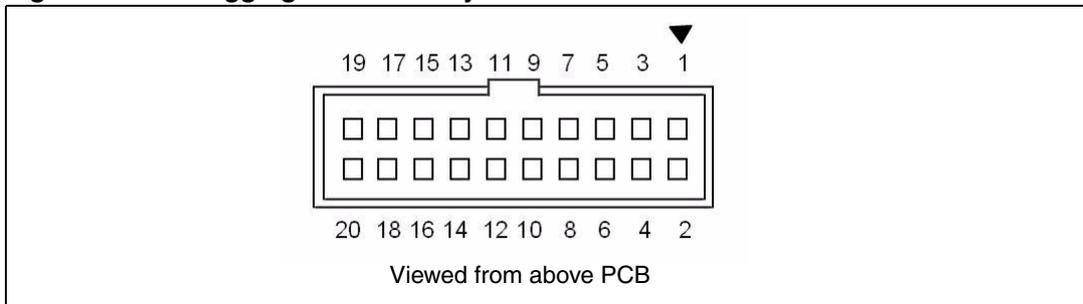
The pinout of the target male connector is given in [Table 3](#).
