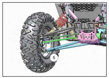
15. Using a soft face hammer, tap on bearing carrier to loosen the lower A-arm ball joint end while pushing downward on the lower A-arm. Completely remove the ball joint end from the bearing carrier.
