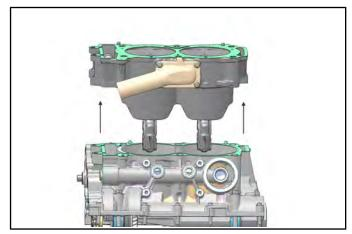
5. Remove the piston / connecting rod assemblies from the cylinder.
