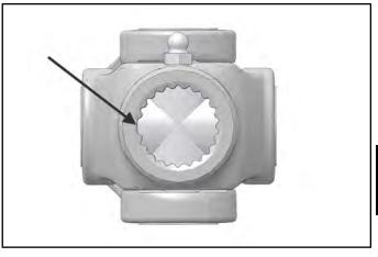
NOTE: Paint marks are applied to the front and rear propshafts to aid shaft alignment. Reference these marks during installation if still visible.
