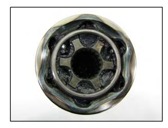
7. Thoroughly clean the joint with an appropriate solvent and dry the joint to prevent any residual solvent from being left in the joint upon reassembly.
