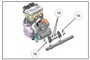
25. With the help of an assistant and the engine hoist, raise the engine vertically out of the vehicle frame.
