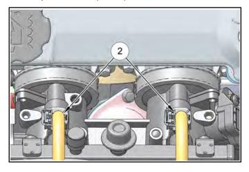
Fuel Injector Resistance Specification: 11.4 - 12.6 Ω
