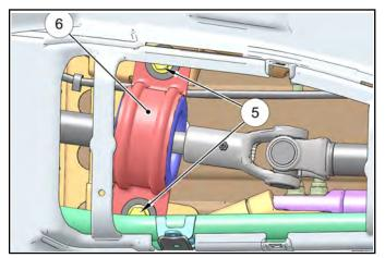
3. While moving the propshaft support bearing assembly, slide the front propshaft off the rear propshaft and remove it from the vehicle.
