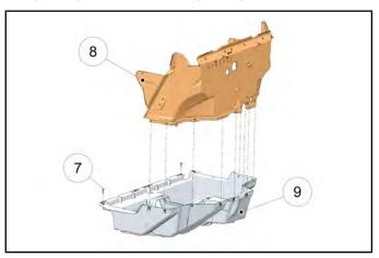
6. Remove the Torx screws (Item 7) retaining the rear portion of the floor and remove the lower floor from the vehicle.
