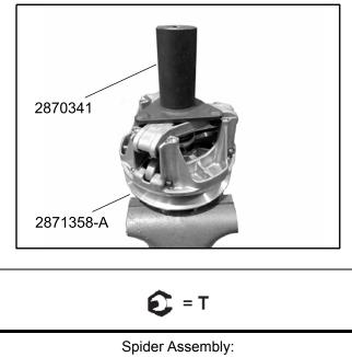
Spider Assembly: 280 - 300 ft-lbs (379 - 406 Nm) Apply 4 mL of Loctite® 620<sup>™</sup> and 4 mL of Loctite® 7088<sup>™</sup> Primer in 90° apart in vertical stripes to the shaft threads.
