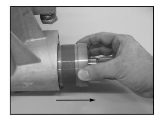
31. Remove the snap ring (Y) and shim (Z) from the snorkel shaft.
