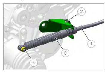
3. If adjustment is required, loosen the lower jam nut (Item 6) and pull the cable out of the mount (Item 2) to move the upper jam nut (Item 5).
