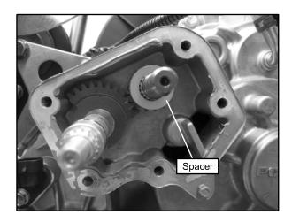
35. Install the detent star onto the shift drum shaft. Be sure to install the detent star with the raised edge facing outward and skip-tooth aligned.
