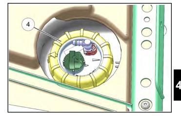
NOTE: Apply downward force on the fuel pump flange while removing the fuel pump PFA nut.
