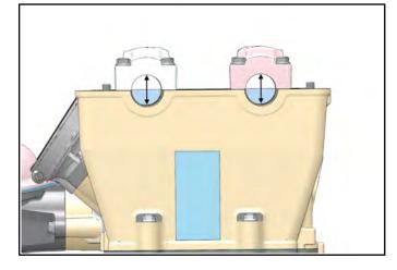
NOTE: Replace cylinder head if camshaft journal bores are damaged or if worn past the service limit.
