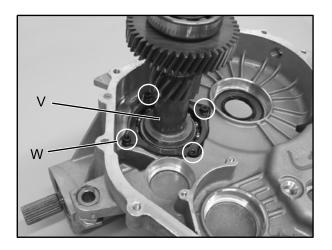
18. Remove all seals from the gearcase halves and clean the cases in preparation for assembly.
