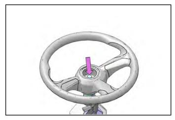
6. Once the steering wheel pops loose, completely remove the nut and lift the steering wheel off the shaft.
