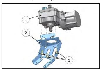
2. Install the power steering unit into the vehicle and align the skip-tooth spline on the power steering stub shaft with the opening in the lower steering shaft.
