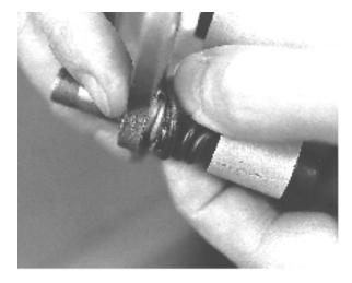
4. Compress the mounting bracket and make sure the dust seals are fully seated. Install the brake pads. Clean the disc and pads with brake parts cleaner or denatured alcohol to remove any dirt, oil or grease.
