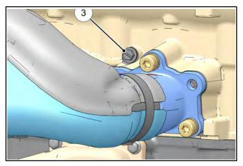
7. Tighten the bleed screw to specification, top off coolant and properly install the pressure cap.
