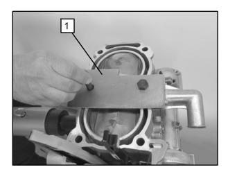
4. Carefully lift the cylinder and pistons from the upper crankcase.
