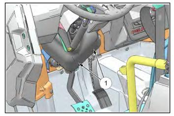
2. Remove the pinch bolt retaining the upper steering shaft to the power steering unit.
