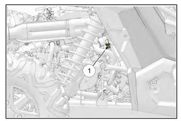
4. Reinstall the dipstick and push it into place. Do not lock the dipstick
