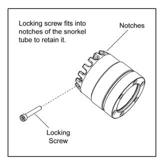
16. Torque the locking screw to specification.
