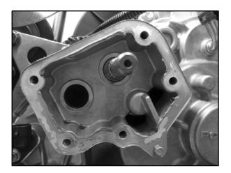
33. Install the sector gear (16T) onto the shift drum shaft. Install the shift shaft assembly and sector gear (11T) into the bushing pocket on the left side. Align the timing marks on the gears as shown.
