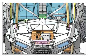
5. Disconnect the instrument cluster, AWD switch, headlight switch, and ignition switch. Note their location and wire routing. Remove the upper dash.
