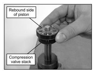
NOTE: If unsure of the valve stack order, refer to "Shock Valving" under the "Shock Service Information" provided earlier in this section.
