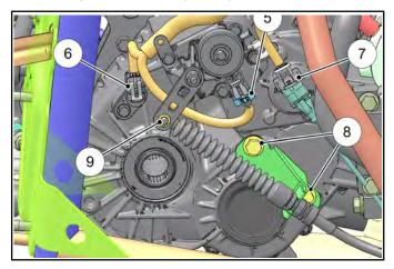
15. Torque the two shift cable bracket bolts to specification.
