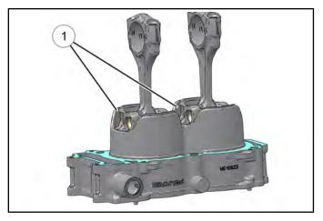
NOTE: Use a slight front to back rocking motion until all rings are captive in cylinder and past the cylinder sleeve opening (Item 1).
