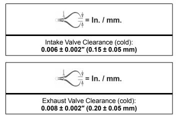
9. If any of the valve clearance measurements are out of specification, remove the camshaft carriers and camshafts and proceed with this procedure.
