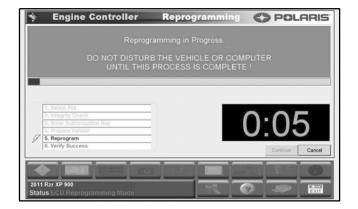
15. Once the ECU reprogramming procedure is complete, click the 'Finish' button on the screen. Verify the reflash was a success by starting the vehicle.
