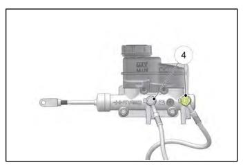
3. Place a container to catch brake fluid under the master cylinder brake line banjo bolts (Item 4).
