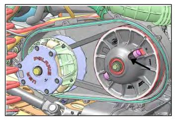
6. Walk the belt out of the driven clutch and drive clutch. Remove the belt from the vehicle.
