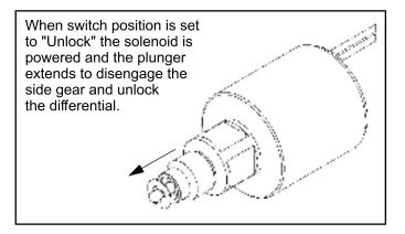
When "Differential-Lock" is selected, power is removed from the electrical solenoid allowing the solenoid plunger to retract. Spring tension moves the shift fork back into place and mates the engagement dog to the side gear that is part of the planetary differential assembly. This locks the rear differential as a solid rear axle, increasing traction.
