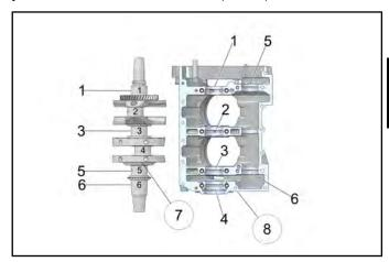
In this example, you would use the number 2 as the crankcase codes (case journals 1, 2, 3, 4). You would use letters G, Y, G, Y as the crankshaft codes (crank journals 1, 3, 5 and 6). Based off the bearing selection chart, you would use:
