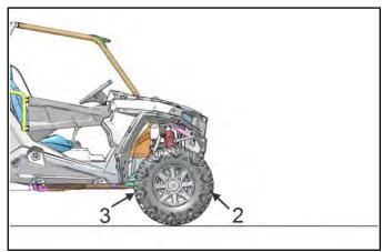
4. Rotate the tires 180° by moving the vehicle forward. Position chalk marks facing rearward, even with the hub/axle center line.
