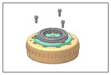
3. Remove the one-way clutch and inspect both sides of drive rollers (Item 1). Inspect the roller contact surface (Item 2) inside the hub for wear, damage or uneven surface.
