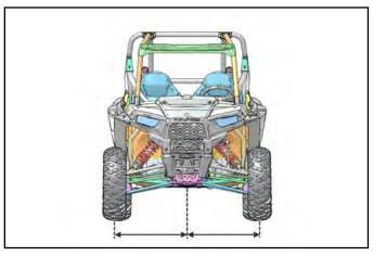
NOTE: Be sure steering wheel is straight ahead before determining which tie rod needs adjustment.
