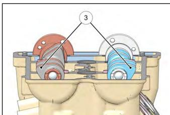
4. Carefully install the rear camshaft carriers onto the camshafts. Carrier openings should face each other when installed properly.
