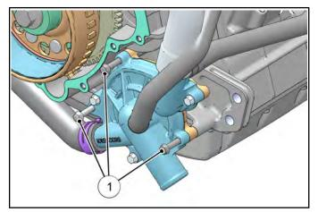
3. Remove the water pump assembly from the engine by using a twisting motion as you pull out on the housing.
