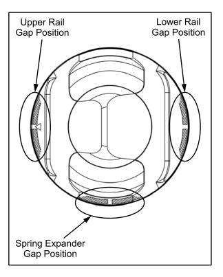
4. Install second ring with marking facing top of piston. Rotate ring to position the end gap toward intake side of piston as shown below.
