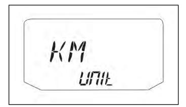
15. Press and hold the MODE button to save the setting and advance to the next display option.
