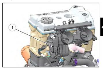
Mounted to the intake plenum, the ETC acts as an electronically controlled throttle body. The ETC controls engine throttle operation to provide the proper air/fuel ratio needed for engine operation at all RPM ranges. The ETC controls engine RPM based off input provided by the Pedal Position Sensor (PPS) and Electronic Control Unit (ECU).
