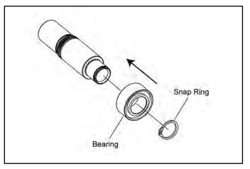
2. Install the shaft and bearing assembly into the outer sheave.
