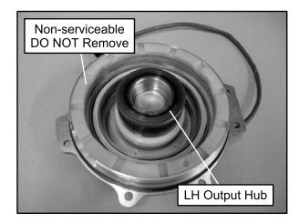
13. Install the output cover assembly onto the gearcase housing. Install the seven cover plate screws and torque to specification.
