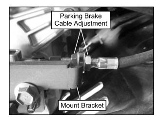
Use two open-end wrenches and loosen the outer jam nut (D). Back out the outer jam nut (D) 1 1/2 turns.
