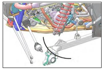
4. Install the lower shock mounting bolt and **new** nut. Torque fastener to specification.
