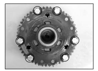
3. Remove the six planet gears and each side gear assembly from the ring gear.
