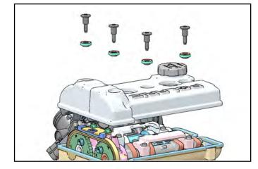
7. The engine will need to be rotated four times to inspect all eight valve clearances (Item 13). Two valves can be measured at each camshaft lobe position.
