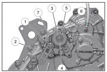
Remove E-clip (Item 3) that retains spring washer (Item 4), flat washer (Item 4) and gear switch (Item 5). Remove the switch. 5. Remove the sector cover bolts (Item 6) and remove the sector cover (Item 7).
