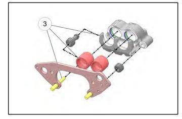
NOTE: Be sure to clean seal grooves in caliper body.
