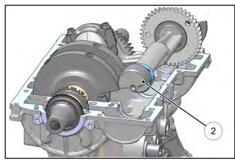
4. Inspect the balance shaft gear teeth for damage.
