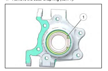
2. From the back side of the bearing carrier, tap on the outer bearing race with a drift punch in the reliefs as shown.
