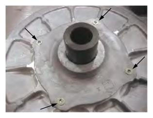
Helix Retaining Screws: 48 in-Ibs (5 Nm)
