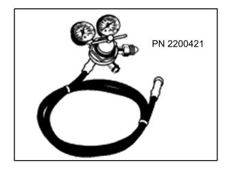
34. Continue filling until the shaft has fully extended and the reservoir pressure is at 200 psi.
