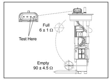
3. Allow the sender float to sit in the **empty position** and compare to specification.
