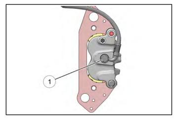
5. Loosen brake pad adjustment set screw 2-3 turns to allow brake pad removal after the caliper is removed.
