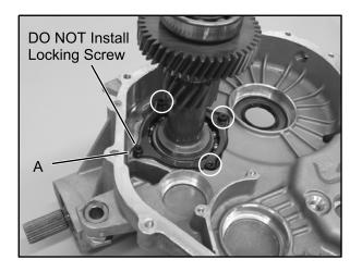
NOTE: DO NOT install the longer screw (A). Installing the longer screw will lock the snorkel tube and not allow for backlash setting adjustment.
