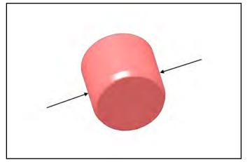
Front Caliper Piston O.D.: Std: 1.370" (34.80 mm) Service Limit: 1.368" (34.75 mm) 3. Inspect the brake disc and pads as outlined in this chapter.
