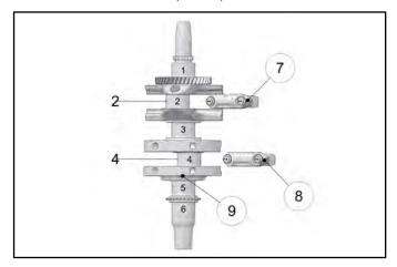
In this example, you would use the number 2 as the connecting rod code. You would use letters *G* and *G* as the crankshaft codes (crank journals 2 and 4). Based off the bearing selection chart, you would use a *Green* bearing for each connecting rod
