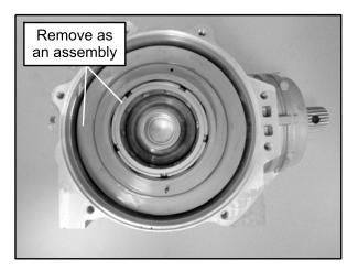
7. Remove the RH output hub assembly from the gearcase housing.
