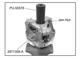
**Clutch Spider Nut Socket: PU-50578** Clutch Holding Fixture: PN 2871358-A 2. Loosen and remove the spider (counterclockwise) using Clutch Spider Removal / Installation Tool (PN 2870341).
