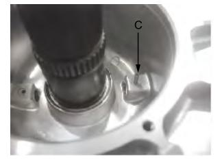
7. Install the spring over the shaft.
