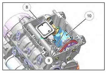
10. Use one of the oil pump retaining bolts or a pen magnet to extract the dowel pins (Item 11) from the oil pump. Doing so allows for oil pump removal without having to remove the pump drive sprocket.
