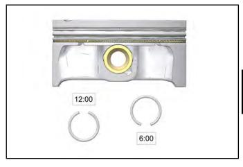
NOTE: Never re-use a piston pin circlip.
