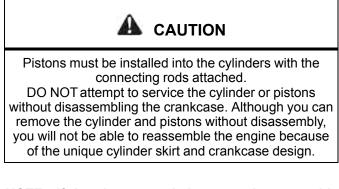
NOTE: If the pistons are being reused, reassemble in the same cylinder bore and direction from which they were removed (MAG / PTO).
