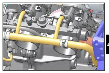
The fuel injectors are non-serviceable. If diagnosis indicates a problem with either injector, test the resistance of the fuel injector(s) by measuring between the two pin terminals (Item 1):
