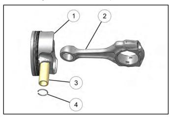
NOTE: Do not tap on pin or cause any sideways force to connecting rod. Warm piston crown with a heat gun if pin cannot be installed by hand, or use a piston pin installation tool.
