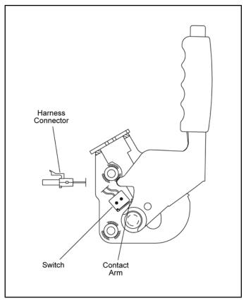
The switch remains in the "open" position when the park brake lever is not applied.
