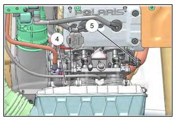
7. Loosen the two hose clamps (Item 6) that retain the dual throttle body assembly (Item 7) to the intake adapters. Carefully lift the throttle body assembly out of the intake adapters.
