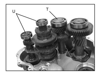
16. Place the gear cluster assembly on a clean surface for inspection. If disassembly is required, refer to "Gear Cluster Disassembly".
