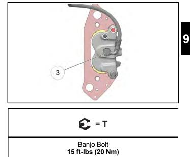
4. Install the adjustment set screw and turn clockwise until stationary pad contacts disc, then back off 1/2 turn (counterclockwise).
