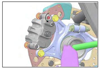
6. Remove the two caliper mounting bolts (Item 2) and remove the caliper assembly from the front hub.
