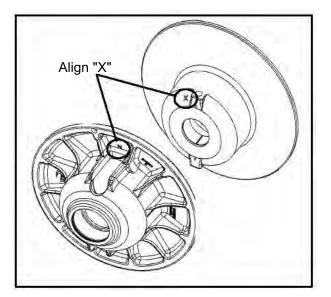
5. Install the roller pin into the sheave assembly on both sides. The flat side of the roller pin faces downward when the shaft side is laying flat on the bench.
