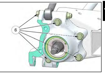
10. Remove the bearing carrier from the rear drive shaft and trailing arm.
