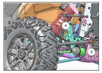
7. Examine A-arm bushings and pivot tube. Replace if worn. Discard hardware.
