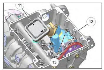
Oil Pump Mounting Bolts: 89 in-Ibs (10 Nm)
