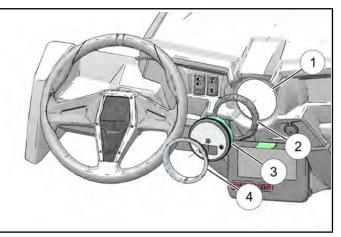
NOTE: Do not remove the rubber mount from the dash panel. Only remove the rubber mount if necessary. The bezel (Item 4) is a snap-on assembly and is a serviceable part.
