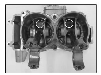
10. Carefully place the cylinder and pistons into the upper crankcase.
