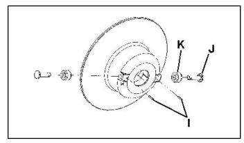
12. Press the shaft and bearing out of the outer sheave using an arbor press.
