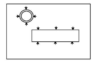
Piston Pin O.D.: 0.7873 - 0.7875" (20.000 - 20.005 mm) Service Limit: 0.7866" (19.98 mm)
