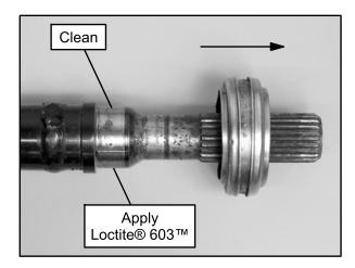
5. Install the new support bearing assembly onto the end of the propshaft.
