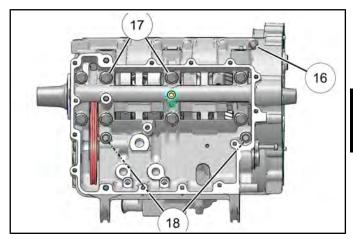
17. Tap on the lower crankcase in reinforced areas with a soft faced hammer to loosen. Carefully lift up and remove the lower crankcase half.
