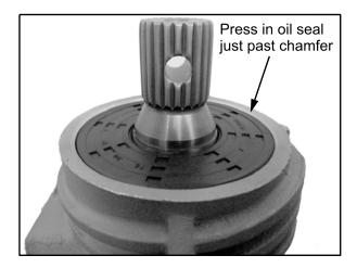
4. Install the RH output hub into the gearcase housing.
