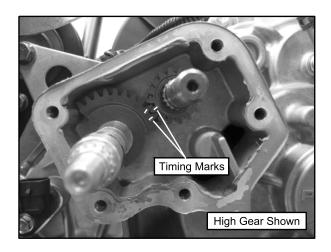
34. Install the spacer onto the shift drum shaft.
