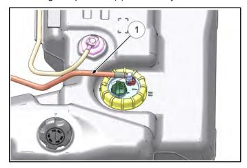
2. Locate the fuel supply fitting (Item 2) through the right rear wheel well on the upper right side of the engine. Check the line and quick-connect fitting for signs of wear, deterioration, damage or leakage. Replace line if necessary.
