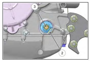
5. Use a shop light to illuminate the water pump drive access hole in engine crankcase and note orientation of the water pump drive slot (Item 3).
