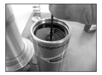
NOTE: When the IFP Tool is removed, the IFP must remain submerged in shock oil to prevent air from getting under the floating piston.
