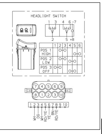
NOTE: Pins 7 and 8 provide power and ground to light the switch lamp.
