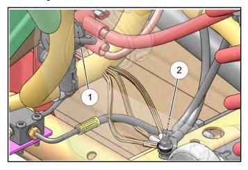
2. Inspect the chassis ground terminals. Be sure the grounds are clean and tight.
