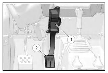
The throttle pedal should move freely and always return back to its idle position when released.
