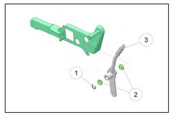
5. Remove both bushings (Item 2) from the shift lever and service as needed.
