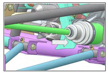
3. Install drive shaft into the front bearing carrier.
