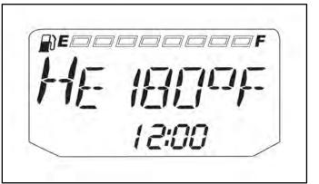
Engine temperature can be displayed in  $^\circ$  F or  $^\circ$  C. Refer to "Units of Measurement" to change the format.
