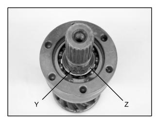
32. Use an arbor press to remove the snorkel tube from the snorkel shaft.
