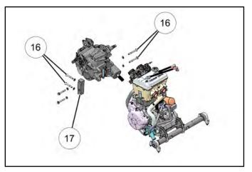
NOTE: It is *not necessary* to remove the bolts that retain the bracket (Item 17) to the transmission.
