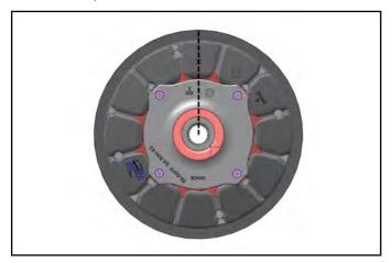
3. Remove the four screws (Item 1) that secure the cam (helix) assembly using a T25 Torx driver.
