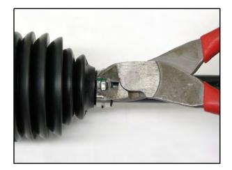
2. Remove the large end of the boot from the plunging joint and slide the boot down the shaft.
