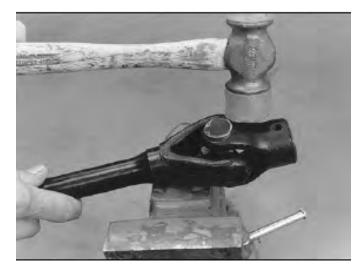
3. Support U-joint in vise as shown and drive inner yoke down to remove remaining bearing caps.
