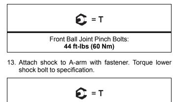
Front Shock Mounting Bolts: 45 ft-Ibs (61 Nm)
