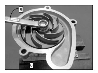
5. Remove impeller from water pump shaft.
