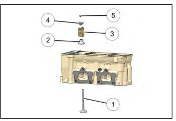
4. Dip the new valve seat/seal (Item 2) in clean engine oil and carefully install the valve seat/seal on the valve guide with a rotating motion. Push firmly until seated in retaining groove and square with the guide
