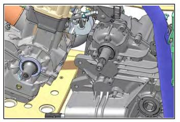
Install the rear transmission mount to the frame and secure with M8 bolts and nuts. Torque nuts to specification.
