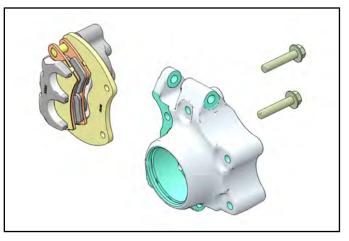
NOTE: When removing caliper, be careful not to damage brake line. Support caliper to avoid kinking or bending brake line.
