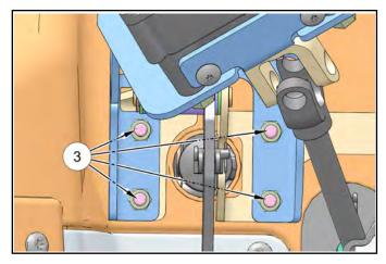
5. Carefully remove the power steering unit and mount bracket from the vehicle as an assembly.
