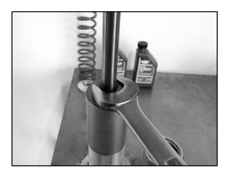
9. Slowly lift up and remove the shock rod assembly from the shock body.
