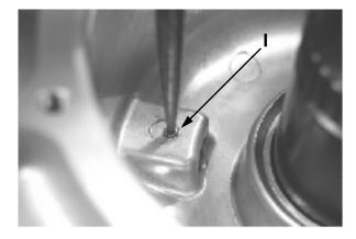
11. Pull out the clutch roller pins (J) and rollers (K).
