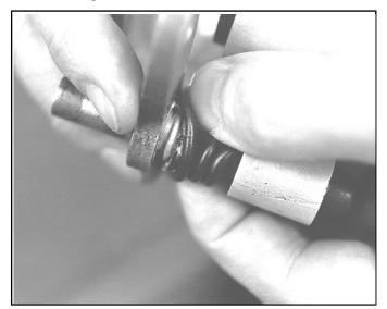
2. Compress mounting bracket and make sure dust boots are fully seated. Install pads with friction material facing each other.
