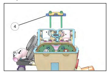
Remove the remaining two bolts that retain the front camshaft carrier (Item 5) and carefully lift the carrier off the camshafts.
