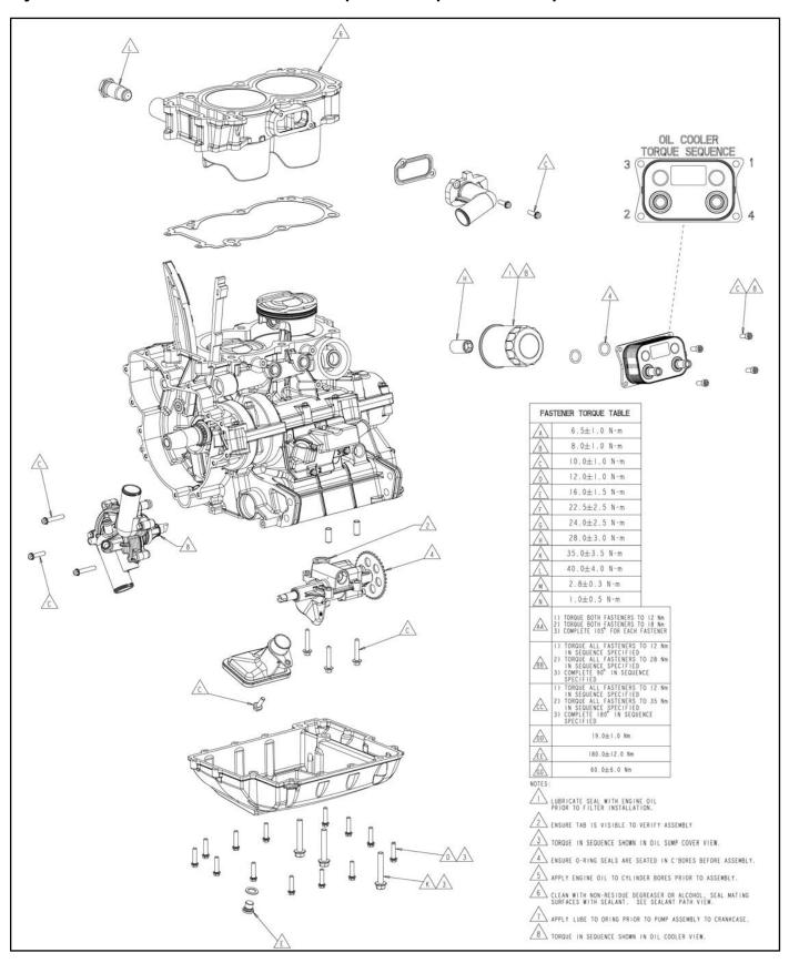
Cylinder / Oil Cooler / Oil Filter / Oil Pump / Oil Sump / Water Pump
