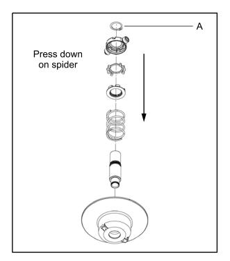
6. Remove the spider assembly and spring (B).
