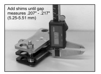
Once you have determined the correct amount of shims to use, reassemble the caliper and apply an Anti-Seize Lubricant to the thrust washer and shims. 4. Torque the caliper assembly bolts to specification.
