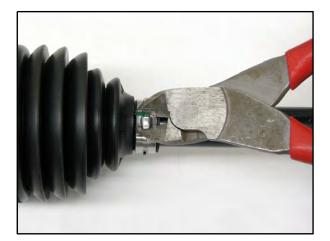
2. Remove the large end of the boot from the CV joint and slide the boot down the shaft.
