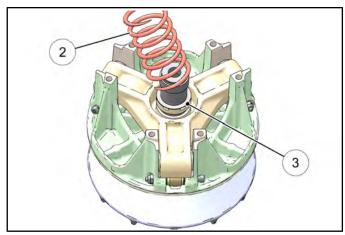
7. Remove and inspect limiter spacer (Item 3). Replace if necessary.
