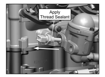
6. Torque the new ECT sensor to specification and connect the vehicle harness to the sensor.
