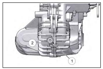
3. If lubricant level is not even with bottom threads, add recommended lubricant as needed. Do not overfill.
