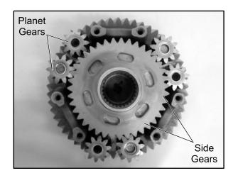
4. Inspect the female side gear (A), male side gear (B), planet gears (C) and ring gear (D). Replace components or bushings as needed. Bushing replacement can be performed on all necessary differential components. If bushing replacement is required, proceed to Planetary Differential Bushing Replacement".
