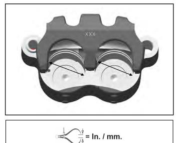
Rear Caliper Piston Bore I.D.: Standard: 1.505" (38.23 mm) Service Limit: 1.507" (38.28 mm)
