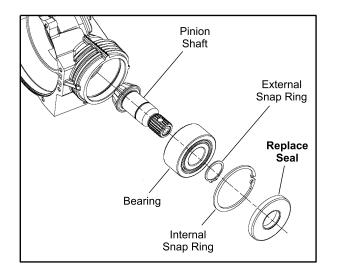
9. Inspect the pinion gear for chipped, broken or missing teeth. Inspect the pinion bearing for signs of wear and the pinion shaft seal surface for pitting.
