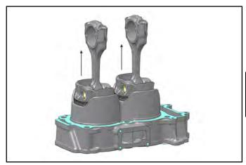
NOTE: If the pistons are to be reused, mark the pistons so they are reassembled in the same cylinder bore and direction from which they were removed (MAG / PTO).
