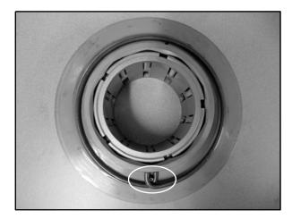
7. Align spring retainer dowel pin with ring gear dowel pin and install the retainer on top of the torsion spring.
