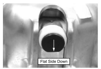
6. Install the spring pins (C) to secure the roller pins. Install until flush with sheave surface.
