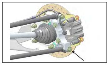
5. Remove the two caliper mounting bolts and lift caliper off the brake disc.
