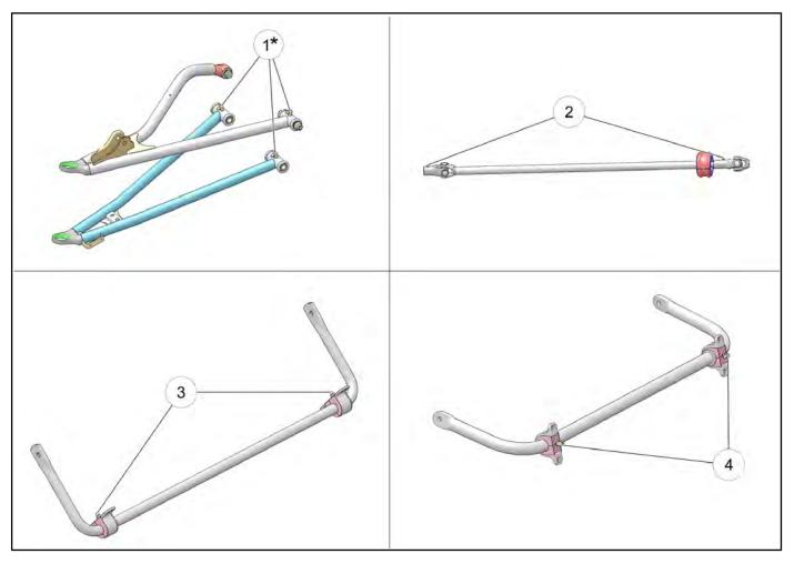
\* there is no grease point on the upper control arm rear mount point
