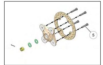
Brake Disc Mounting Bolts (Item 5): 30 ft-Ibs (41 Nm)
