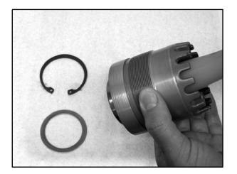
35. Remove the retaining ring to remove the remaining washer, bearing and gear from the snorkel shaft.
