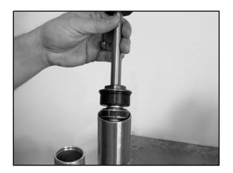
10. Remove and properly dispose of the oil from the shock body.
