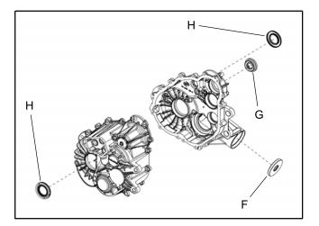
28. Thoroughly clean the shift shaft housing. Be sure the transmission is in High gear prior to reassembly.
