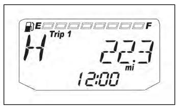
The trip meter records the miles traveled by the vehicle on each trip. To reset the trip meter:
