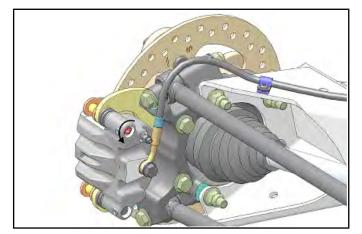
4. Remove the lower radius rod outer mounting bolt, nut and washer from the bearing carrier. Swing radius rod down. Discard the nut.
