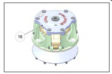
12. Install cover bolts and torque in a cross pattern evenly to specification.
