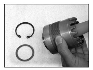
32. Remove the retaining ring to remove the remaining washer, bearing and gear from the snorkel shaft.
