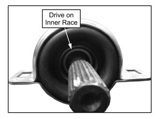
NOTE: Take care while installing the support bearing assembly. Be sure to only drive on the inner race of the bearing. Driving on the bearing or support in any other location will damage the bearing or support assembly.
