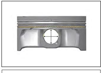
Piston Pin Bore I.D.: 0.7877 - 0.7881" (20.009 - 20.018 mm) Service Limit: 0.7893" (20.05 mm)
