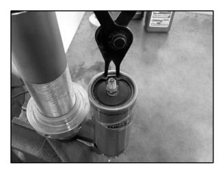
7. Carefully remove the cap from the reservoir body.
