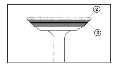
Intake Seat Cutter Diameter: 1.567" (39.80 mm)
