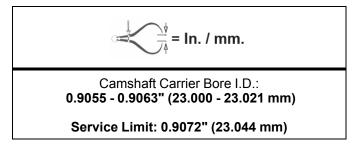
Calculate oil clearance by subtracting camshaft journal O. D. s from camshaft carrier bore I. D. s. Compare to specification.
