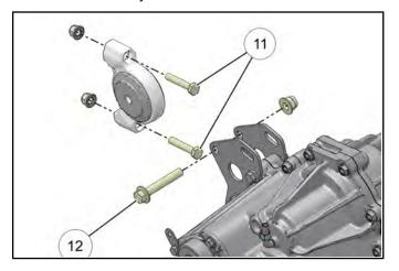
23. Slide transmission towards the rear of the vehicle. Lift and rotate the top of the transmission towards the left side of the vehicle. With the help of an assistant, remove transmission from the left rear wheel well area.
