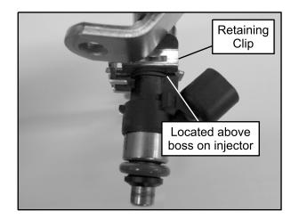
NOTE: Be sure the retaining clip is positioned on the injector and fuel rail as shown above.
