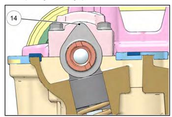
9. Measure the valve clearance using a feeler gauge.
