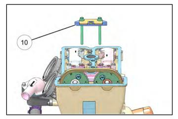
20. Torque the camshaft carriers bolts in sequence to specification.
