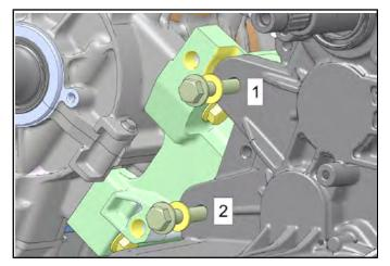
11. Torque right side mounting bolts to specification using the numbered sequence shown.
