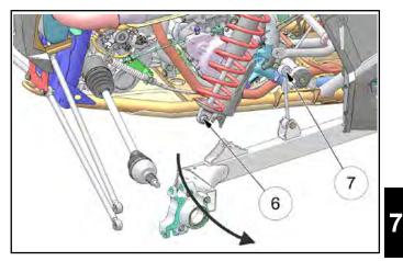
14. With a short, sharp jerk, remove drive shaft from the transmission splines.
