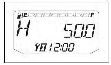
The initial factory service interval setting is 50 hours. Each time the engine is started, the engine hours are subtracted from the service interval hours. When the service interval reaches 0, the LCD wrench icon will flash for approximately 10 seconds each time the engine is started.
