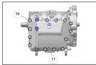
24. Torque the oil sump cover bolts in sequence to specification. Repeat the sequence to verify final torque.
