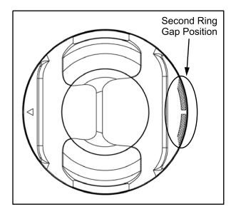
5. Install top ring with mark facing top of piston. Rotate ring to position the end gap toward exhaust side of piston as shown below.
