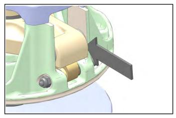
**Button to Tower Clearance:** .000-.012 (.000-.304 mm)
