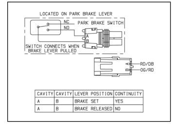
Apply the parking brake. Continuity should now exist between the switch terminals. If no continuity exists when the parking brake is applied, try to clean the switch terminals and re-test. Replace switch if necessary.
