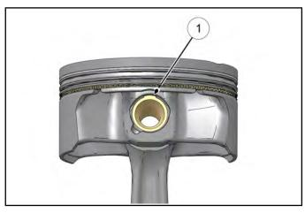
2. Remove piston circlip and push piston pin out of piston. If necessary, heat the crown of the piston slightly with a heat gun if pin cannot be removed by hand. Discard circlips.
