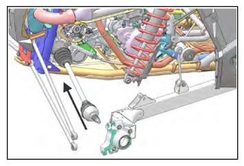
3. Swing the rear trailing arm assembly outward and upward until the rear axle can be inserted into the bearing carrier. Support the trailing arm from underneath.
