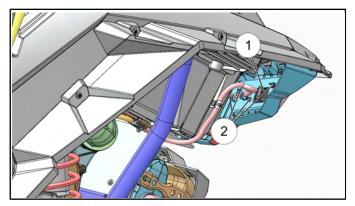
2. While holding the taillight assembly, remove the three nuts (Item 2) retaining the taillight assembly and remove it from the rear fascia.
