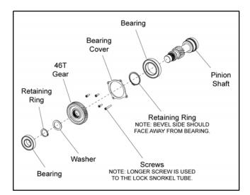
NOTE: If pinion shaft was disassembled, the bearing cover must be installed on the shaft before installing the 46T gear.
