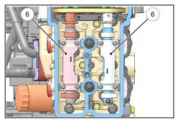
Install the Cylinder Holding & Camshaft Timing Plate (PU-50563) into the end of camshafts as shown. Use a 13/16" open-end wrench to rotate camshafts slightly if needed.
