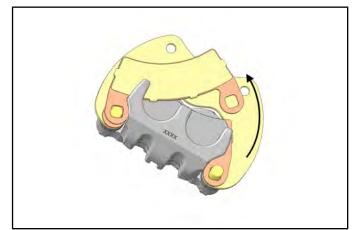
8. Remove the inner brake pad.
