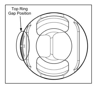
6. Be sure top and second rings rotate freely in their grooves and do not bind when compressed by hand.
