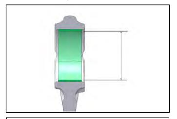
Connecting Rod Small End I.D.: 0.7879 - 0.7885" (20.015 - 20.030 mm) Service Limit: 0.7897" (20.06 mm)
