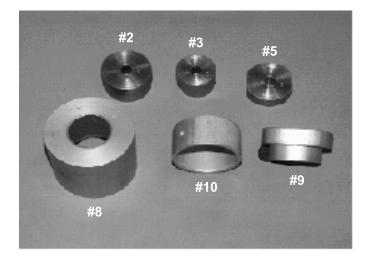
NOTE: Bushings are installed at the factory using Loctite® 609. In order to remove bushings it will be necessary to apply heat evenly to the area around each bushing. Clean all residual Loctite® from bushing bore prior to installing new bushing.
