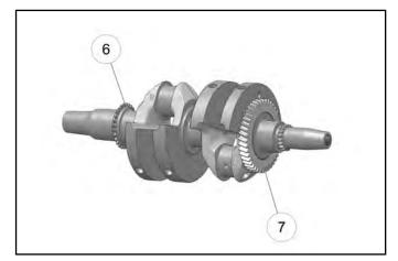
8. If the crankshaft gear or sprocket is damaged, the crankshaft assembly must be replaced.
