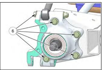
9. Remove the bearing carrier from the rear drive shaft and trailing arm.
