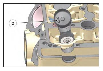
2. Compress the valve spring by hand using valve spring compressor adapter (PV-43513-A).
