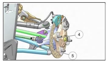
8. Torque the tie rod end fastener (Item 5) to specification and install a **new** cotter pin (Item 5).
