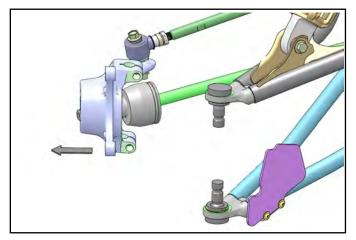
10. With a short, sharp jerk, remove drive shaft from the front gearcase.
