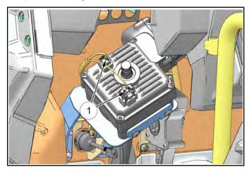
3. Remove the pinch bolt retaining the lower steering shaft to the power steering unit.
