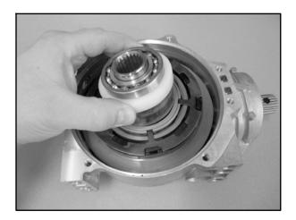
NOTE: Nylon spacer is non-serviceable and should not be removed.
