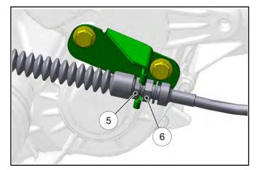
Adjust the shift cable so there is the same amount of cable travel when shifting slightly past HIGH gear and PARK. 5. Thread the upper or lower jam nut as required to obtain proper cable adjustment.
