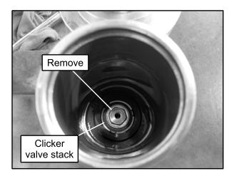
NOTE: Keep the valve stack in the order it was removed. If unsure of order, refer to "Shock Valving" under the "Shock Service Information" provided earlier in this section.
