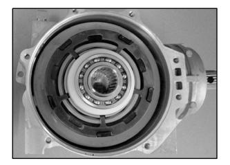
11. Install a new O-ring on the cover plate assembly.
