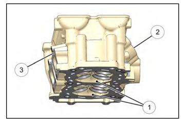
3. Repeat for exhaust valves by pouring fluid into each exhaust port (Item 3).
