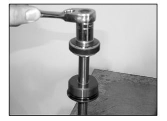
NOTE: Keep the rebound and compression valve stacks in the order they were removed. If unsure of order, refer to "Shock Valving" under the "Shock Service Information" provided earlier in this section.
