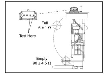
Fuel Sender Resistance Specifications: Full:  $6 \pm 1 \Omega$ Empty:  $90 \pm 4.5 \Omega$
