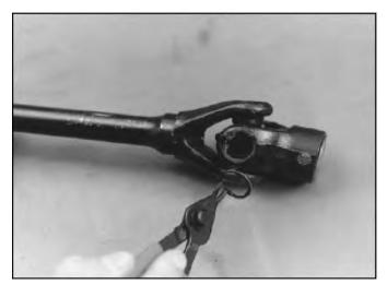
NOTE: If yoke or bearing is removed, cross bearing must be replaced. Note orientation of grease fitting and mark inner and outer yoke for correct re-positioning during installation.
