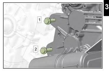
12. Torque right side mounting bolts to specification using the numbered sequence shown.
