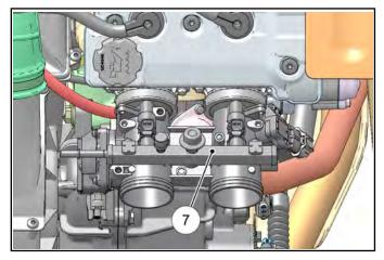
10. Pull out on the fuel injector retaining clip and pull the injector out of the fuel rail. Repeat on the other injector if removal is necessary.
