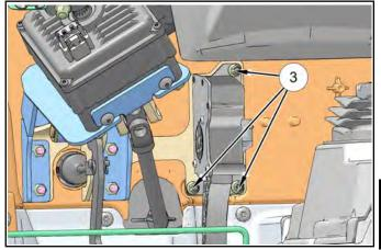
4. Remove the pedal assembly from the vehicle.
