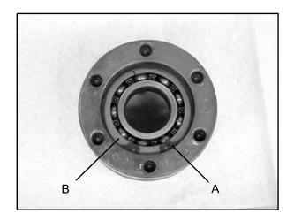
31. Lightly tap on the bearing from the opposite side to remove it from the snorkel tube.
