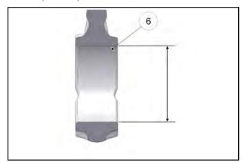
8. Refer to the number stamped onto the exhaust side of the connecting rod. This number represents the bore diameter.
