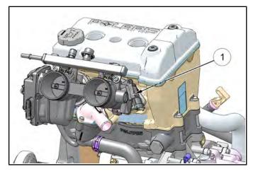
These sensor signals, comprised of separate intake air temperature and manifold absolute pressure readings are processed by the ECU and compared to its programming for determining the fuel and ignition requirements during engine operation. The T-MAP provides the ECU with engine load data.
