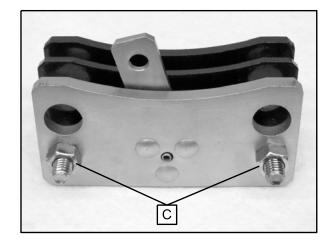
2. Slide the brake pads and springs from the assembly.
