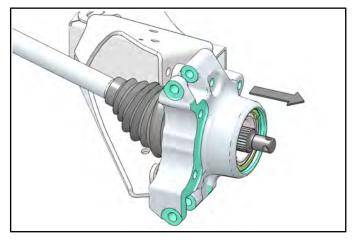
11. Rotate bearing by hand and check for smooth rotation. Visually inspect bearing for moisture, dirt, or corrosion.
