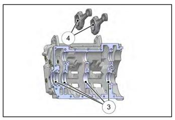
NOTE: Always replace plain bearings when the crankcase or connecting rods have been disassembled. Refer to "Bearing Selection Chart".
