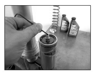
6. Using a snap ring pliers, remove the retaining ring from the reservoir.
