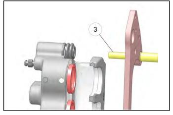
Compress the mounting bracket and make sure the dust seal boots are fully seated. Install the brake pads. Clean the disc and pads with brake parts cleaner or denatured alcohol to remove any dirt, oil or grease.
