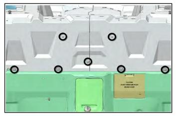
10. Remove the cargo box half from the vehicle.
