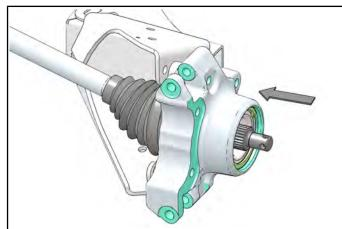
2. Install the four fasteners (Item 1) that attach the rear bearing carrier to the trailing arm. Install the (1) fastener (Item 2) that attaches the upper radius rod to the bearing carrier. Torque bolts to specification.
