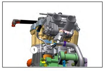
Coolant passes through the thermostat housing and by the sensor probe, varying a resistance reading which is relayed to the ECU. This signal is processed by the ECU and compared to its programming for determining the fuel and ignition requirements during operation. The ECU also uses this signal to determine when to activate the cooling fan during operation.
