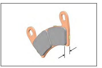
Front Brake Pad Thickness: 0.297 ± 0.007" (7.5 ± .178 mm) Service Limit: 0.180" (4.6 mm)
