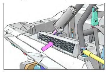
3. Inspect the pre-filter. If necessary, clean with soapy water and dry with low pressure compressed air.
