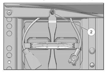
5. Lift the battery out of the vehicle.
