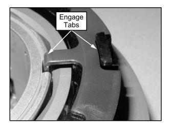
NOTE: Verify armature plate tabs are in the roll cage slots and that it rests properly on the spring retainer.
