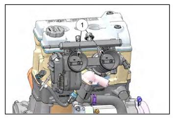
The throttle body assembly also includes the Electronic Throttle Control and Idle Air Control.
