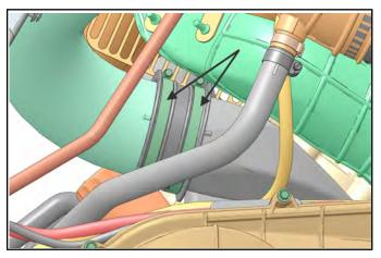
13. Loosen hose clamps (Item 3) that attach clutch outlet duct to inner clutch cover. Disengage hose from the cover.
