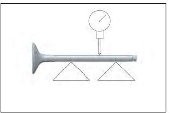
3. Check the end of the valve stem for flaring, pitting, wear or damage.
