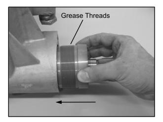
5. Install the snorkel shaft into the gearcase. Using the Snorkel Tool (PA-50231), tighten the snorkel tube until it is lightly seated in the transmission housing.
