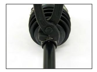
Axle Boot Clamp Tool: PU-48951 or CV Boot Clamp Pliers: 8700226
