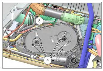
14. Remove the seven bolts (Item 4) that retain inner clutch cover to engine and transmission. Remove inner clutch cover.
