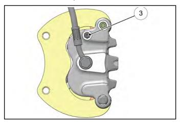
NOTE: Do not release foot pedal before bleeder screw is tight or air may be drawn into master cylinder.
