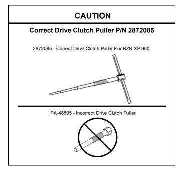
NOTE: Be sure to use the correct Drive Clutch Puller (PN 2872085) to prevent damage to crankshaft.
