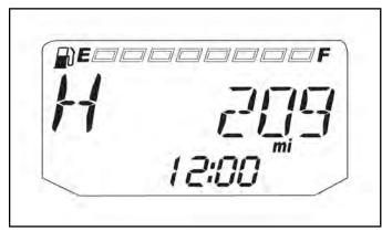
The odometer records and displays the total distance traveled by the vehicle. The odometer can not be reset.
