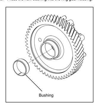
4. Install the bushing to the specified depth as shown.
