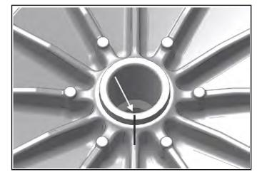
NOTE: Upon reassembly, if the reference marks created in step 2 are not in alignment, the clutch will not be in balance and the assembly MUST be replaced.
