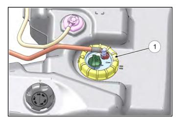
NOTE: Neither filter is serviceable individually. Must replace the fuel pump as an assembly.
