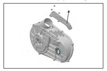
12. Loosen the hose clamp attaching PVT inlet duct to the inner clutch cover. Disengage the hose from the inner clutch cover.
