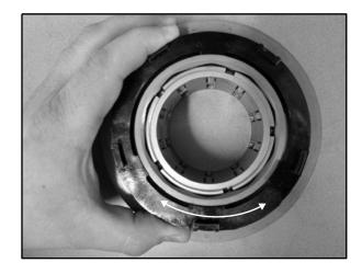
9. Install armature plate. Be sure all of the armature plate tabs are fully engaged into the roll cage assembly and that it is resting properly on the torsion spring retainer.
