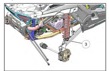
16. Place a spacer or support between the vehicle frame and engine to hold the engine up in position.
