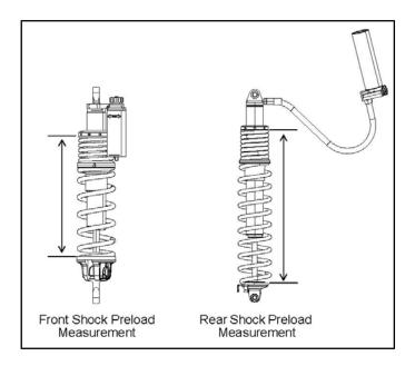
NOTE: Always return the spring preload to the factory setting after the load is removed from the vehicle. The increased suspension height will negatively impact vehicle stability when operating without a load.
