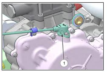
A ferromagnetic 35-tooth encoder ring with a missing tooth is built onto the flywheel. The inductive speed sensor is mounted  $1.0 \pm 0.26$  mm ( $0.059 \pm 0.010$  in.) away from the encoder ring. During rotation, an AC pulse is created within the sensor for each passing tooth. The ECU calculates engine speed from the time interval between the consecutive pulses.
