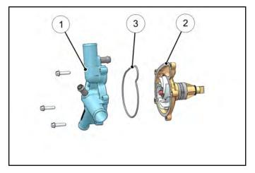
20. Install the water pump cover and three retaining bolts (Item 8). Torque bolts in sequence to specification.
