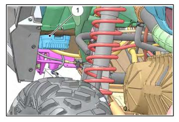
NOTE: If the regulator / rectifier case temperature exceeds 230° F or 110° C, the unit will turn itself off to cool down. The unit will turn on again after it has cooled down to at least 212° F or 100° C. If it turns off, verify the cooling fins are clean, free from debris and that adequate airflow is present.
