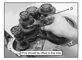
NOTE: Shift fork pins should be offset towards the input shaft as shown above.
