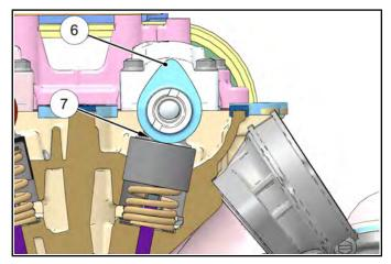
Measure the valve clearance (Item 7) using a thickness (feeler) gauge. Record the measurement if clearance is out of specification.
