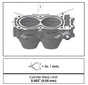
2. Inspect cylinder for wear, scratches, or damage.
