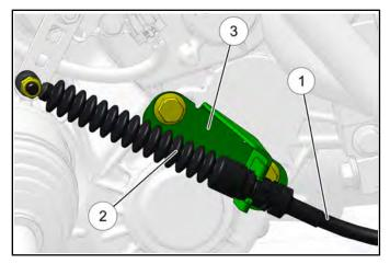
3. If adjustment is required, loosen the lower jam nut (Item 4) and pull the cable out of the mount (Item 3) to move the upper jam nut (Item 5).
