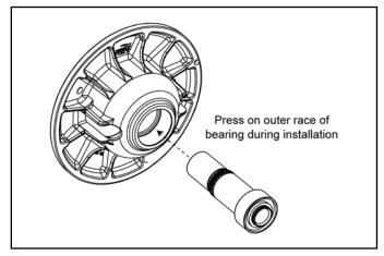
NOTE: Press only on the outer race of the bearing during installation to prevent damaging the bearing.
