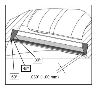
Exhaust Seat Cutter Diameter: 1.364" (34.65 mm)
