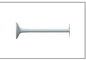
4. Inspect split keeper groove for wear or flaring in the keeper seat area.
