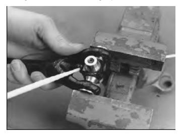
3. Using a suitable arbor, fully seat the bearing cap in one side. Continually check for free movement of bearing cross as bearing caps are assembled.
