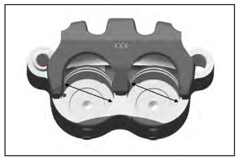
Front Caliper Piston Bore I.D.: Std: 1.373" (34.87 mm) Service Limit: 1.375" (34.93 mm)
