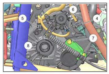
19. Remove the wire ties retaining harness to transmission and mounts.
