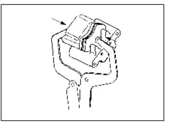
NOTE: Brake fluid will be forced through compensating port into master cylinder fluid reservoir when piston is pushed back into caliper. Remove excess fluid from reservoir as required. 7. Push caliper mounting bracket inward and slip outer brake pad past the edge to remove.
