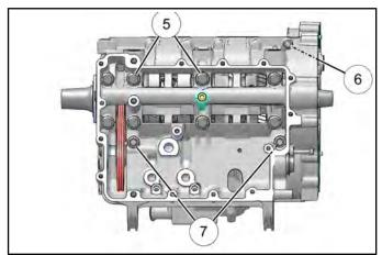
NOTE: Install new M10 lower crankcase bolts.
