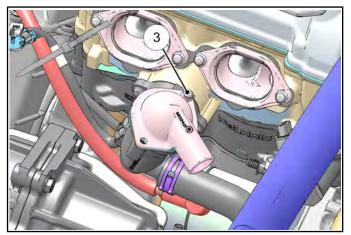
8. Lift the cover from the housing and remove the thermostat.
