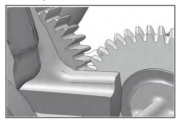
3. Carefully rotate the balance shaft (Item 2) and remove it from the crankcase.
