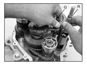
14. Remove the shift shaft rail (Q) and shift forks from the transmission housing as an assembly.
