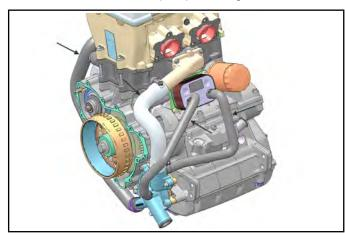
2. Remove the three long gold colored bolts retaining the water pump housing to the engine.
