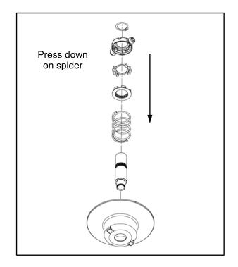
13. Slowly compress the spider into place. If the spider appears to bind while compressing, stop and make sure the skip-tooth on the shaft and the spider are aligned. Once the spider passes the retaining ring notch on the shaft, install the retaining ring.
