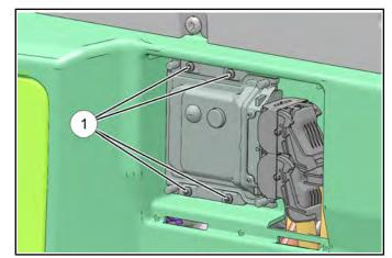
3. With the ignition turned off, disconnect the wire harness from the ECU. Lift the connector locking lever and rotate it up until the connector is free from the ECU.
