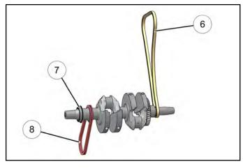
9. Carefully lower the crankshaft into upper crankcase. Guide connecting rods onto the rod journals of crankshaft as necessary.
