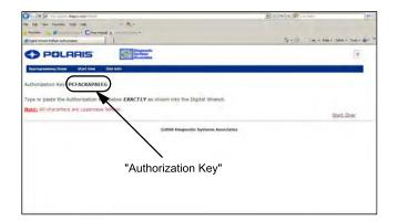
Enter or paste (CTRL +V) the Authorization Key in the box located on the Digital Wrench® screen. Click the 'Continue' button and follow instructions provided on the screen to complete reprogramming procedure.
