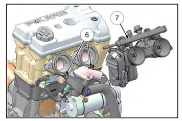
8. Remove the two screw retaining the fuel rail to the throttle body. Lift the fuel rail and injectors out of the throttle body assembly taking care not to damage the fuel injector ends.
