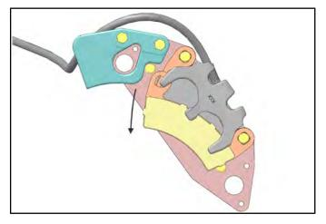
7. Remove the inner pad from the bracket and caliper.
