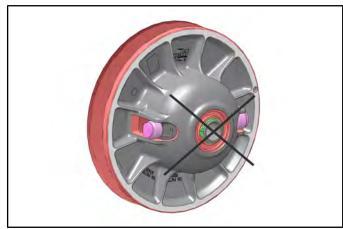
2. It is important to mark the position of the shaft, cam cover and sheave before disassembly or use the X's on the components for reference. This will aid in assembly and maintains clutch balance.
