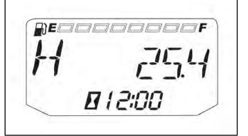
Engine hours are logged anytime the engine is running. Total hours can not be reset.
