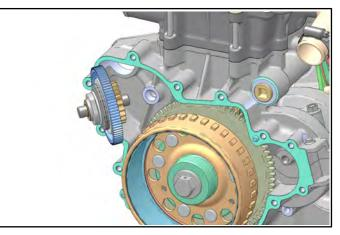
Inspect gear teeth for damage. Inspect fit of shaft inside gear and replace gear assembly is clearance is excessive. Inspect the shaft and bearing surfaces in the crankcase and stator cover for excessive wear.  Using a commercially available strap wrench (Item 1), hold the flywheel and remove the flywheel retaining bolt (Item 2).
