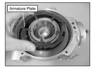
5. Remove the torsion spring retainer and torsion spring from the top of the ring gear.
