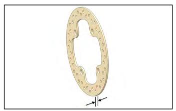
Brake Disc Thickness New: .0188" (4.78 mm) Service Limit: 0.170" (4.32 mm)
