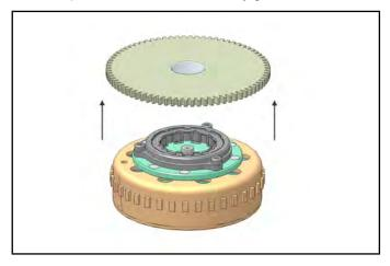
2. Remove the three one-way clutch retaining screws.
