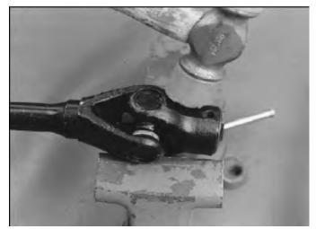
7. When installation is complete, yokes must pivot freely in all directions without binding. If the joint is stiff or binding, tap the yoke lightly to center the joint until it pivots freely.
