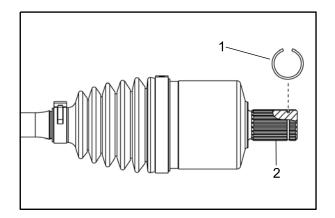
2. Align splines of drive shaft with front gearcase and reinstall the drive shaft. Use a rubber mallet to tap on the outboard end of the drive shaft if necessary
