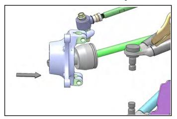
4. Install the upper and lower ball joint ends into the front bearing carrier.
