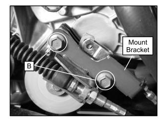
3. Lift the parking brake caliper off the brake disc and remove it from the vehicle.
