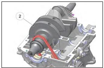
6. Remove the cam chain (Item 3), oil pump drive chain (Item 5) and PTO main seal (Item 4) from the crankshaft.
