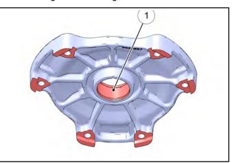
Cover Bushing Inspection: Replace the cover bushing if more brass than Teflon™ is visible on the bushing. Refer to bushing replacement in this chapter.
