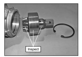
10. Inspect the AWD coil located in the outer cover plate assembly. Refer to "AWD Diagnosis" for detailed inspection process. Replace the cover plate seal and O-ring.
