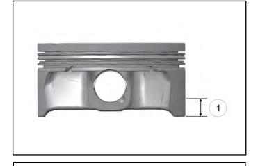
Piston O.D. (Standard): 3.6597 ± 0.0003" (92.959 ± 0.008 mm) Piston to Cylinder Clearance:
