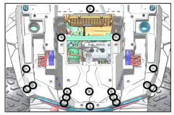
9. Remove the seven T-40 Torx screws on the cab side of cargo box.
