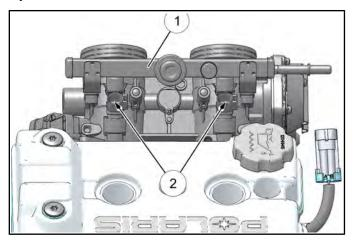
When the key switch is on, the fuel rail is pressurized, and the EFI relay provides voltage to the injectors. During engine operation, the ECU completes the ground circuit, energizing the injectors. The valve needle in each injector is opened electromagnetically, and the pressure in the fuel rail forces fuel down through the inside. The "director plate" at the tip of the injector contains a series of calibrated openings which directs the fuel into the intake port in a cone-shaped spray pattern.
