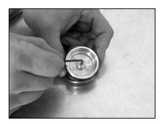
17. Pull IFP up until its top is approximately 1" (2.54 cm) from top of reservoir and remove the IFP Tool. Using a 3/32" Allen wrench, install the IFP bleed screw.
