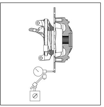
Brake Disc Runout: Service Limit: 0.010" (0.254 mm)
