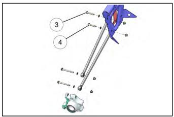
6. Remove radius rods from vehicle.
