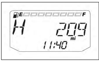
The clock displays the time in a 12-hour or 24-hour format. Refer to "Units of Measurement" to change the format (Standard 12-hour / Metric-24 hour). To set the clock, follow these steps:
