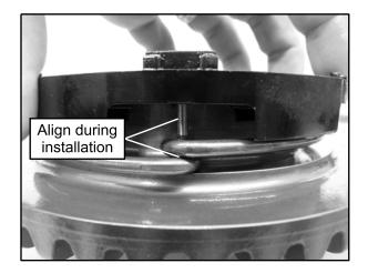
8. Check the action of the torsion spring by rotating in both directions to ensure the spring and retainer are installed properly.
