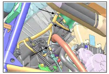
20. Using a 15mm socket, remove the four bolts from the left side (Item 9) and right side (Item 10), securing the transmission to the engine.
