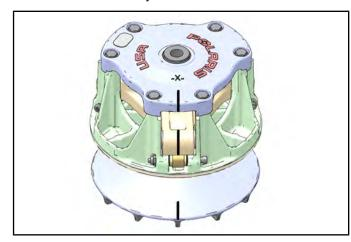
Mark the stationary sheave and clutch shaft to verify the shaft has not rotated in the sheave after tightening the spider during clutch assembly.
