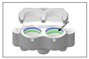
6. Clean the caliper body, pistons and retaining bracket (Item 3) with brake cleaner or alcohol.
