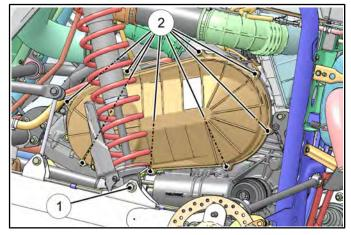
11. Remove drive belt, drive clutch, driven clutch, inner clutch cover and clutch outlet duct (see Chapter 6).
