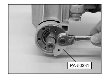
6. Inspect the pinion shaft assembly. Replace bearings if needed. Inspect each gear for damage, chips or abnormally worn teeth.
