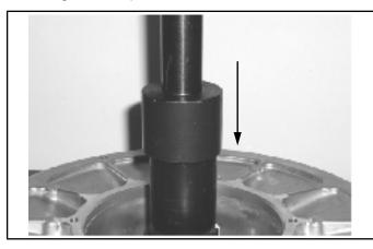
13. Inspect the bearing for wear. Spin the bearing, if the bearing does not spin smoothly, replace it. To replace the bearing, remove the snap ring from the end of the shaft and press the bearing off the shaft.
