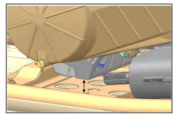
14. Install and properly route the gear position switch connector (Item 5), speed sensor connector (Item 6), crankshaft position sensor connector (Item 7), shift bracket and shift bracket bolts (Item 8), shift cable clevis pin and washer (Item 9) onto the transmission.
