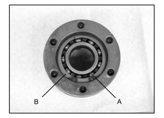
34. Lightly tap on the bearing from the opposite side to remove it from the snorkel tube.
