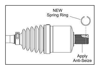
2. Align splines of drive shaft with transmission splines and reinstall the drive shaft. Use a rubber mallet to tap on the outboard end of the drive shaft if necessary.
