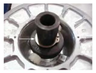
14. Install the cam (helix) assembly over the shaft. Line up the "X" on the cam, "X" on spider, and "X" on the stationary sheave or use the marks previously made before disassembly. **NOTE:** If the cam assembly (helix) is difficult to install, be sure the sheaves are aligned. To align the sheaves place the clutch assembly on a flat surface with the cam assembly (helix) side down. Press down on the moveable sheave belt face with both hands and the helix will release.
