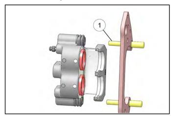
2. Compress mounting bracket and make sure dust boots are fully seated. Install pads with friction material facing each other.
