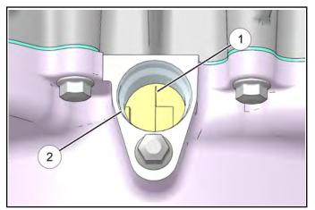
NOTE: DO NOT use the "V" mark located on the flywheel opposite of the "I" mark. Only the "I" mark should be used as a TDC reference.
