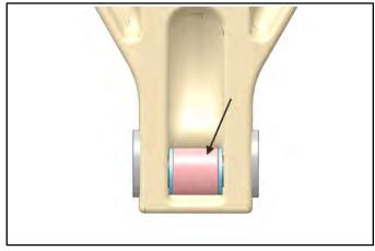
NOTE: Rollers, pins, thrust washers and buttons are not serviceable at the time of this publication.
