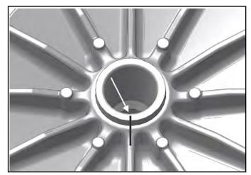
10. Install the limiter spacer (Item 15) and the clutch spring (Item 14).
