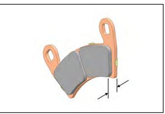
Rear Brake Pad Thickness: 0.298 ± 0.007" (7.57 mm ± .178 mm) Service Limit: 0.180" (4.6 mm)
