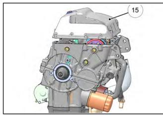
23. Install the thirteen M6 (Item 16) and three M8 bolts that retain the oil sump cover (Item 17) to the crankcase.
