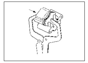
NOTE: Brake fluid will be forced through compensating port into master cylinder fluid reservoir when piston is pushed back into caliper. Remove excess fluid from reservoir as required.
