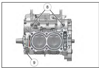
13. Torque the upper crankcase bolts in sequence to specification (start with #12). Repeat the sequence to verify final torque.
