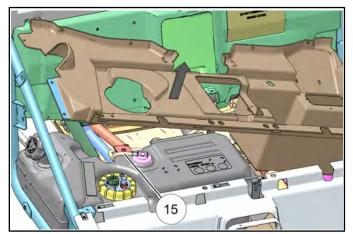
14. Lift the rear of the fuel tank up first. Carefully pull the fuel tank out of the vehicle.
