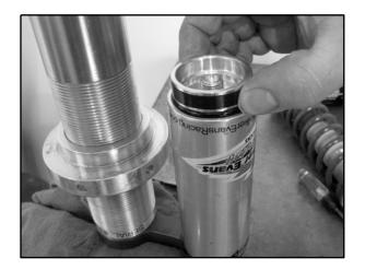
15. Screw IFP Tool (PS-45908) onto the floating piston.
