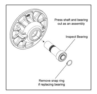
14. Inspect the cam (helix) assembly bushing for wear. If the bushing is worn or the shaft does not fit snug into the bushing, replace the cam (helix) assembly.
