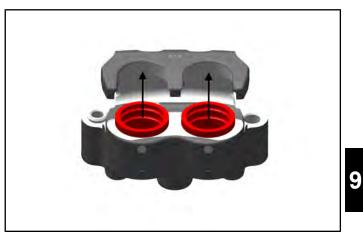
NOTE: Do not remove the caliper pistons with a standard pliers. The piston sealing surfaces will become damaged if a standard pliers is used.
