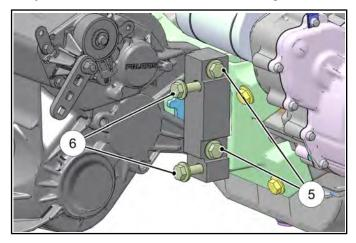
9. Align the front transmission mounting holes with transmission joint bracket mounting holes on engine.
