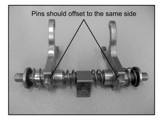
NOTE: Both shift forks need to be orientated the same way, so that the shift fork pins are both offset to the same side of the rail.
