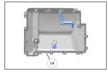
22. Install the oil sump cover (Item 15) onto the crankcase.
