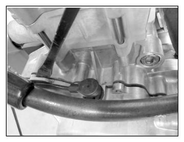
3. Inspect the condition of the stator windings (Item 1) and output wires (Item 2). If replacement is required, refer to Chapter 10.
