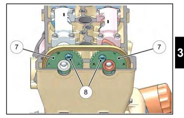
NOTE: Use new sprocket retaining bolts upon assembly.
