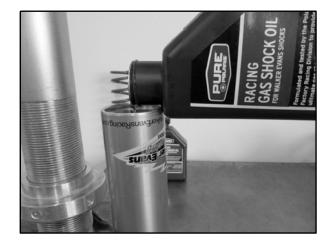
14. Apply a thin film of oil to IFP O-ring and wear band. Insert IFP into reservoir until completely submerged. Allow air to escape as you install the piston.
