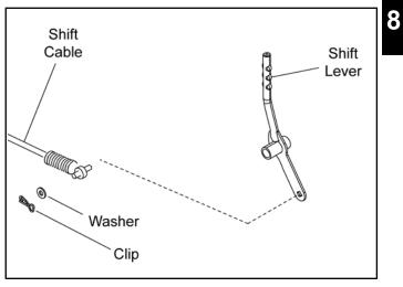
4. Remove the retaining ring (Item 1) and slide the shift lever (Item 3) off the mounting bracket and out from the frame.
