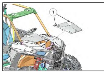
2. Lift rear of hood and slide forward to disengage the front tabs and remove the hood from the vehicle.
