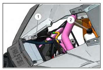
With the engine at operating temperature, the coolant level should be between the upper and lower marks on the coolant recovery bottle. If not, perform the following procedure:
