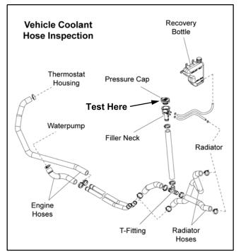
3. The system must maintain 10 psi for five minutes or longer. If pressure loss is evident within five minutes, check the filler neck, radiator, hoses, clamps and water pump weep hole for leakage.
