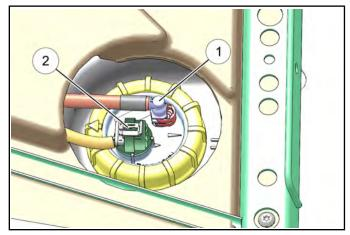
NOTE: A small amount of fuel may come out of the fuel lines or pump fitting. Properly drain fuel into a suitable container.
