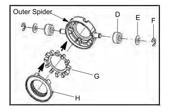
10. Install the spider assembly onto the shaft with the retaining ring on top of the spider. **NOTE:** Use the marks previously made to align the skip tooth spider, or use the "X" on top of the spider and align it with the skip tooth on the shaft.
