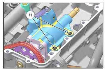
NOTE: If unable to extract the dowel pins from the oil pump, the oil pump sprocket must be removed. Access the sprocket bolt by removing the case plug.
