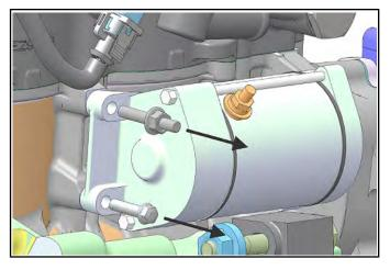
NOTE: The (-) negative battery cable is mounted to the engine using the upper starter mounting bolt / stud.
