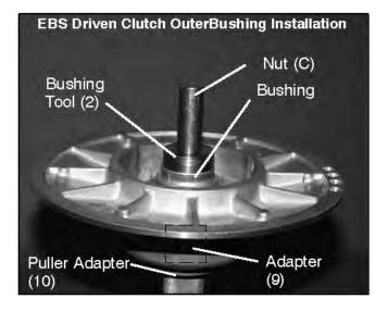
13. Apply Loctite® 609 evenly to bushing bore inside moveable sheave.
