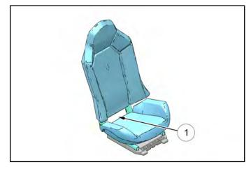
2. Lift upward and forward on the seat while lifting up on the latch lever and remove the seat from the vehicle.
