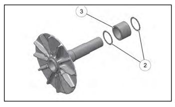
4. Inspect surface of shaft for pitting, grooves or damage. Measure the outside diameter and compare to specifications. Replace the drive clutch assembly if shaft is worn or damaged.
