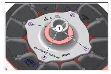
4. Place the driven clutch into the Universal Clutch Compressor **PU-50518**.
