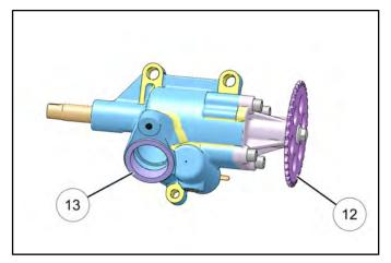
NOTE: Oil pump assembly is non-serviceable
