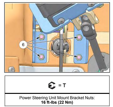
6. Proceed to "Upper Steering Shaft Installation (EPS Models)" to complete the installation procedure.
