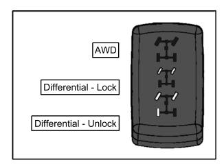
When "Differential-Unlock" is selected, the rear differential becomes unlocked for tighter turns. An electrical solenoid mounted in the rear portion of the gearcase actuates the shift fork. The solenoid plunger extends out to move the fork and slides the engagement dog away from the side gear that is part of the planetary differential assembly. This unlocks the rear differential. The rear drive shafts are now dependent on the differential allowing for tighter turns.
