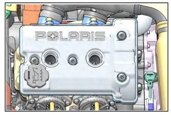
6. Remove the four T40 bolts retaining the valve cover.
