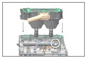
11. Install the Cylinder Holding & Camshaft Timing Plate (PU-50563) onto the cylinder. The cylinder holding tool retains the cylinder and pistons when the engine is rotated.
