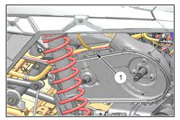
5. Install the protective cover and the four push rivets that secure the cover to the top of the inner PVT cover.
