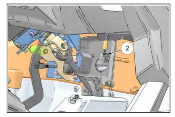
2. Remove the drivers seat and disconnect the negative (-) battery cable.
