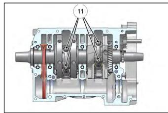
14. Torque connecting rod bolts to specification.
