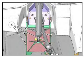
4. Remove the steering shaft, pivot tube and steering wheel from the vehicle as an assembly.
