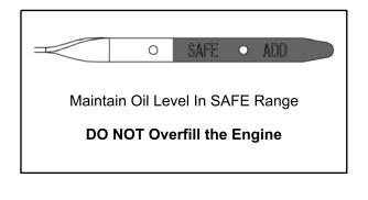
NOTE: A rising oil level between checks during cold weather operation can indicate contaminants such as gas or moisture collecting in the crankcase. If the oil level is over the upper mark, change the oil immediately.
