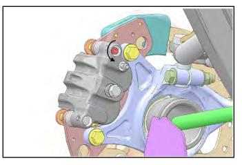
4. Remove the upper and lower caliper mounting bolts and remove the caliper from the front hub.
