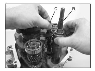
13. Remove the shift shaft rail (Q) and shift forks from the transmission housing as an assembly.
