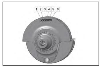
13. Use the table below to see if the crankshaft bearing journals are within specification. If worn past the service limit, replace the crankshaft assembly.
