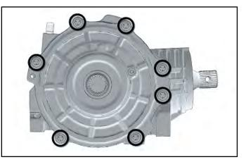
3. Remove the LH output hub assembly from the clutch housing or outer cover plate assembly.
