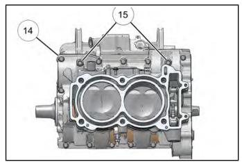
15. Rotate the engine so the cylinder is facing down.
