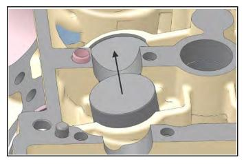
NOTE: Keep mated parts together and in order with respect to their location in the cylinder head for assembly purposes. Mark each component or place them in an organized rack as you remove them. 11. Record the 3 digit number on the bottom of the tappet. (Item 8).
