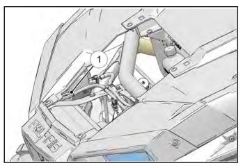
3. The pressure cap relief pressure is 13 psi. Replace cap if it does not meet this specification.
