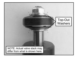
9. **Front Shocks Only:** Assemble the clicker valve stack on top of the fastener and install the assembly into the reservoir body. Tighten the valve stack fastener securely.
