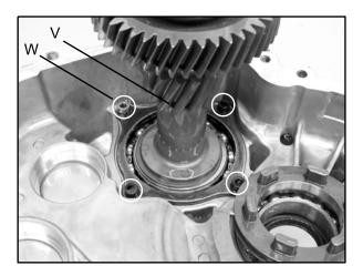
21. Remove all seals from the gearcase halves and clean the cases in preparation for assembly.
