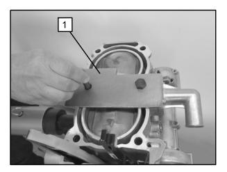
NOTE: Once the cylinder head is removed, nothing retains the cylinder to the engine. DO NOT rotate the engine without using the Cylinder Holding & Camshaft Timing Plate (PU-50563).
