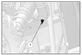
2. Check the drain to ensure it is not plugged with debris so it can drain properly. If needed, remove the drain from the baffle box during inspection.
