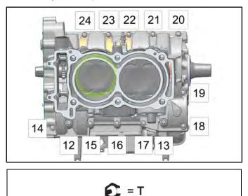
Upper Crankcase Bolts: M8 Bolts: **26 ± 1 ft-lbs (35 ± 2 Nm)** M6 Bolts: **89 ± 9 in-lbs (10 ± 1 Nm)**
