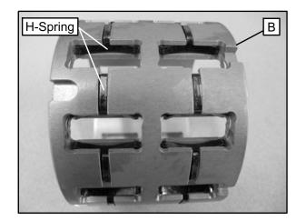
15. Inspect both output hub assemblies. Inspect the bearings and replace if needed.
