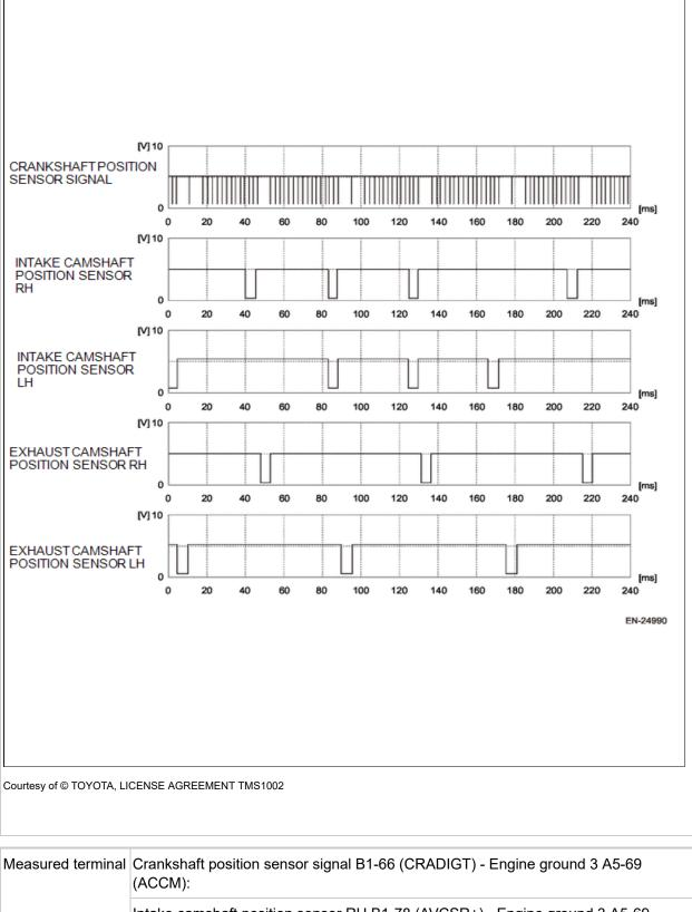
Intake camshaft position sensor RH B1-78 (AVCSR+) - Engine ground 3 A5-69 (ACCM):
