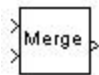
Figure 1.26.46: The Merge block combines its inputs into a single output line whose value at any time is equal to the most recently computed output of its driving blocks. The Merge block often is used to merge a calculation signal with a reset signal.
