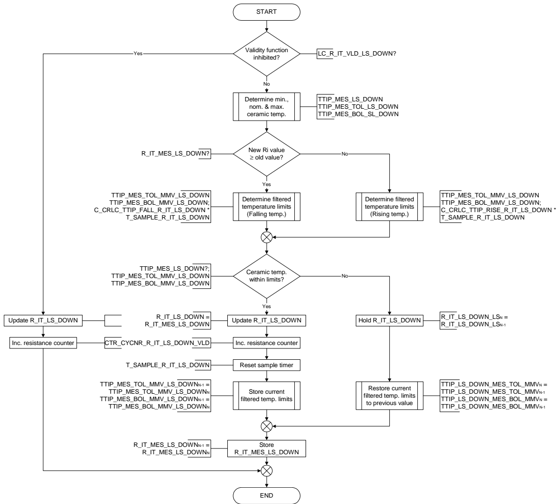
Figure 4.40.4: Function flow chart, Internal resistance validity determination
