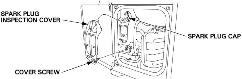
3. Remove the spark plug cap.
