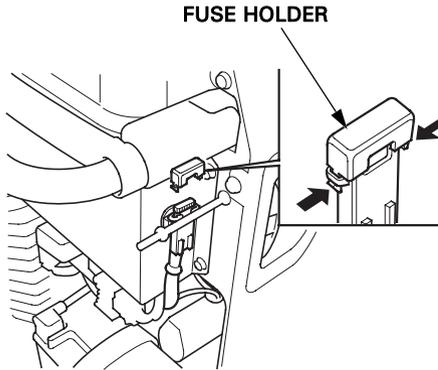
If frequent fuse failure occurs, determine the cause and correct the problem before attempting to operate the generator further.
