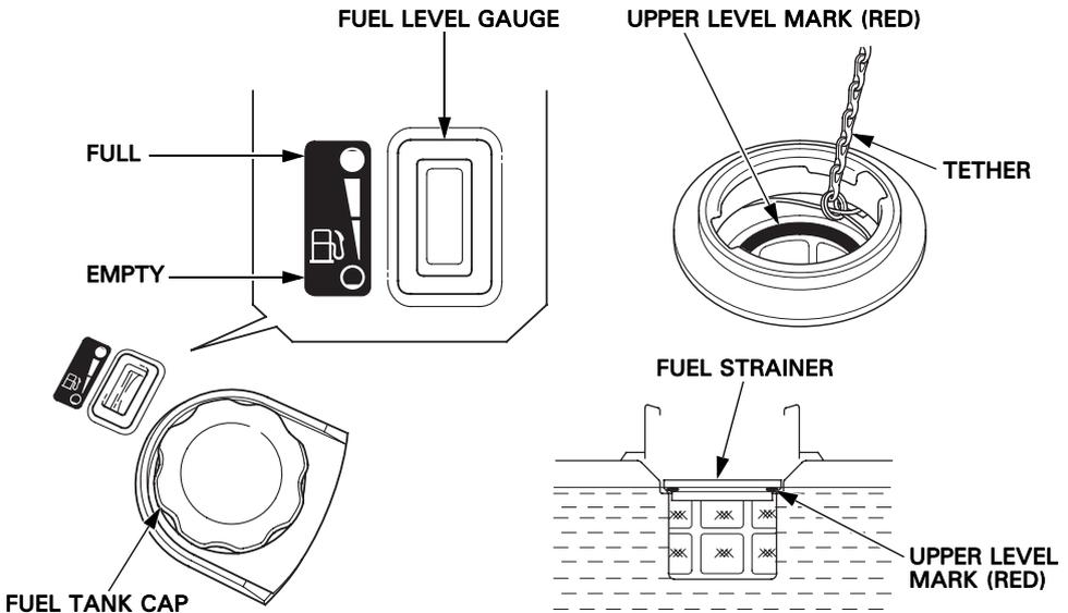
After refueling, reinstall the fuel tank cap securely.
