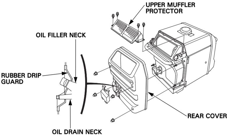
When installing the rear cover, carefully fit the rubber drip guard around the oil filler neck and oil drain neck.
