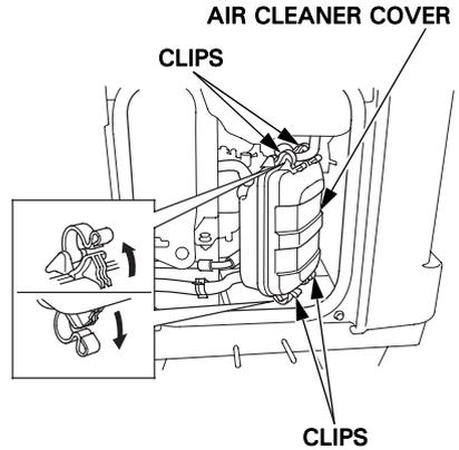
3. Check the foam air filter and paper air filter to be sure they are clean and in good condition. If the foam air filter is dirty, clean it as described on page 48. Replace the foam air filter if it is damaged. If the paper air filter is dirty, replace it with a new one. Do not clean the paper air filter.
