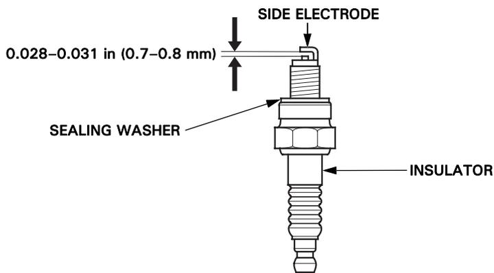
8. Check that the spark plug sealing washer is in good condition, and thread the spark plug in by hand to prevent cross-threading.
