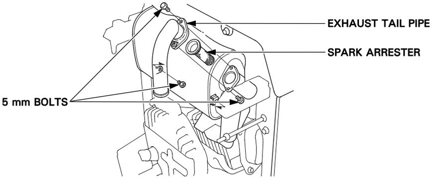
7. Use a brush to remove carbon deposits from the spark arrester screen.
