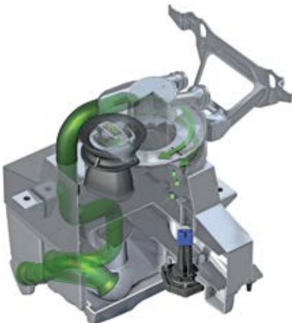
Oil tank with dry sump lubrication
