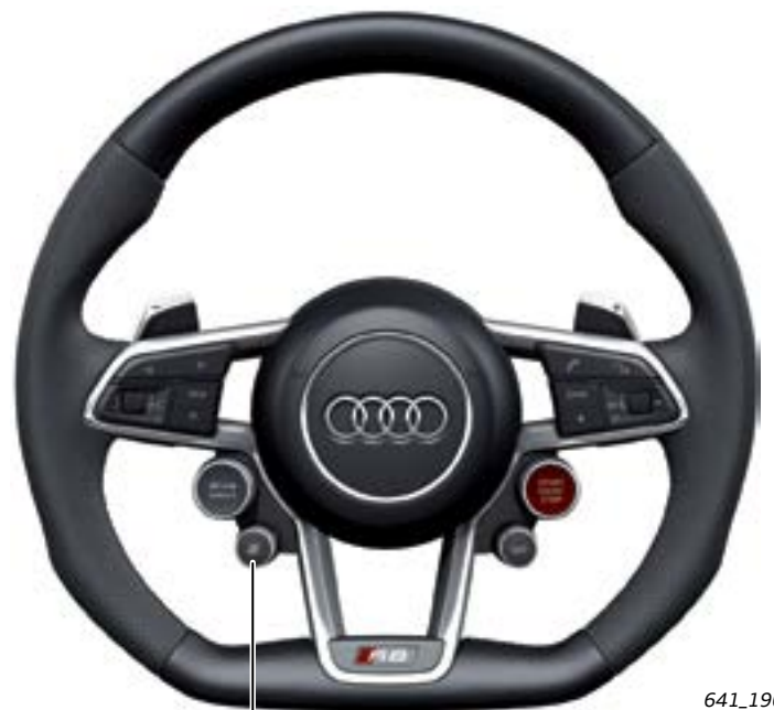
Performance button with adjusting ring for selecting the snow , wet and dry modes
