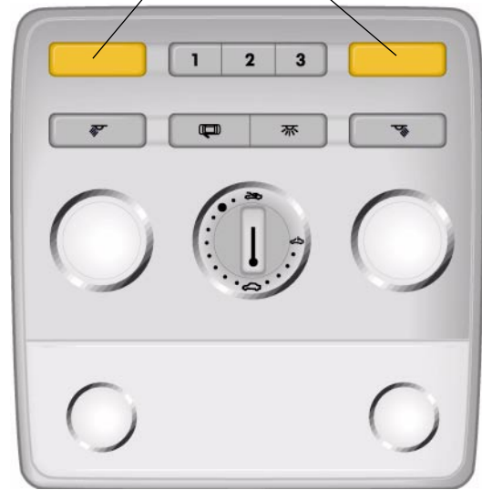
Front roof module
