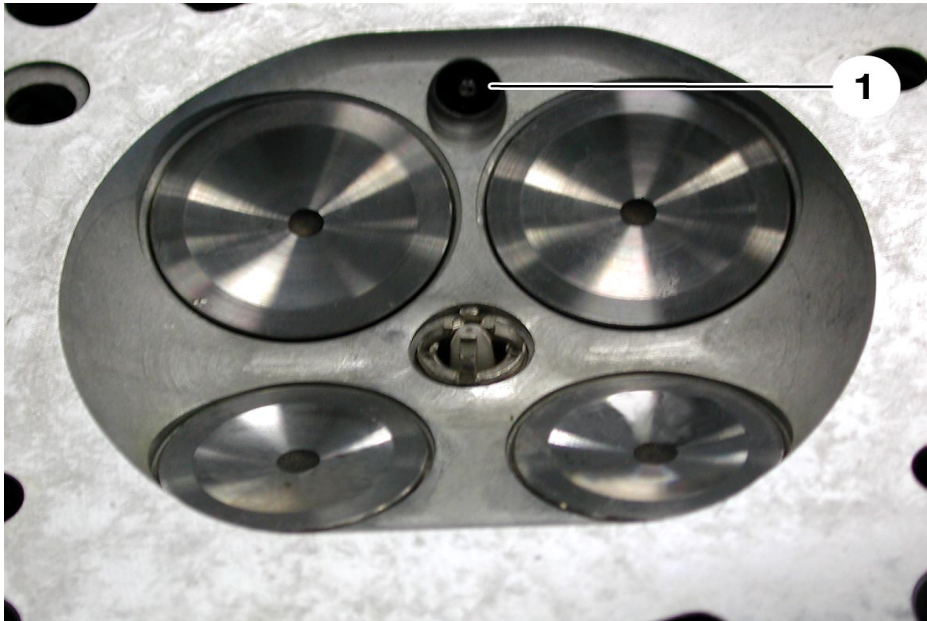
Fig. 42: Position of fuel injector (1) in cylinder head
