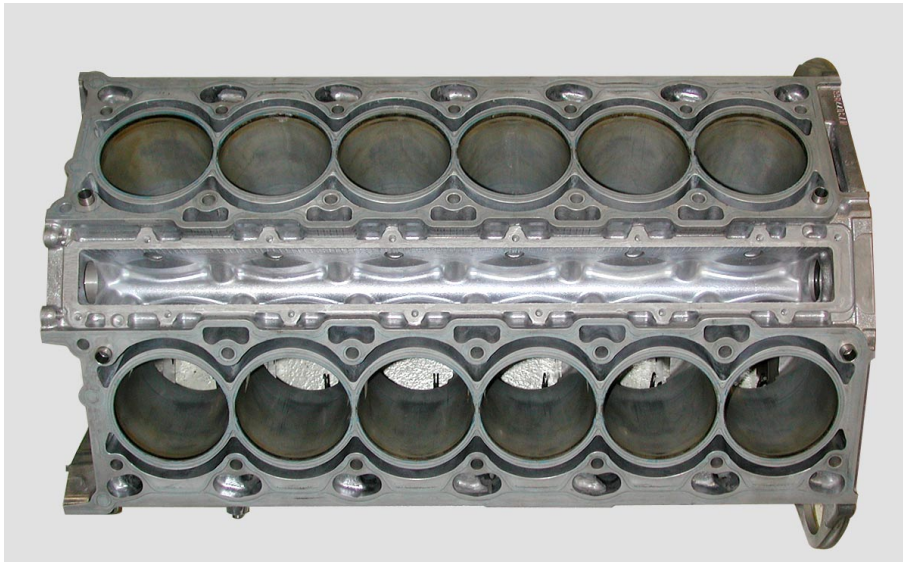
Fig. 31: Aluminium engine block
