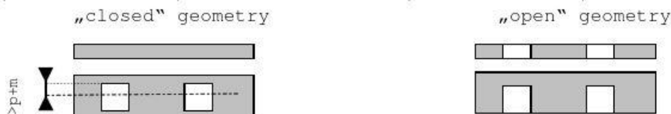
Figure_13: Inadmissible tone wheel geometry (m: displacement from the middle of the tooth, p: pole core diameter)
