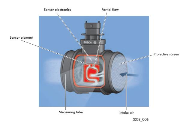
If dirt particles, engine oil vapour and humidity reach the sensor element, the measuring result will be incorrect. For this reason, particular attention was paid to ways of stopping these impurities reaching the sensor electronics when the measuring tube and the protective screen were designed.
