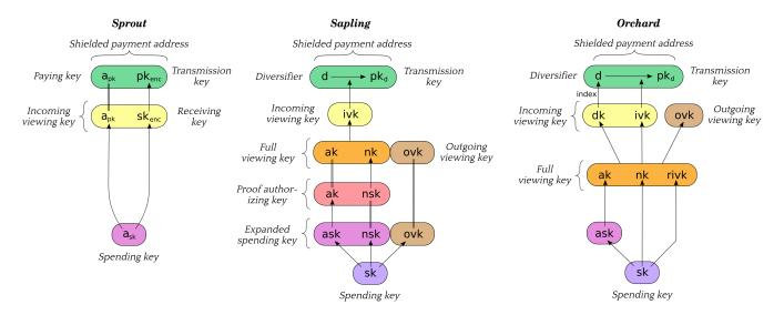
**[Sprout]** The receiving key  $sk_{enc}$ , incoming viewing key  $ivk = (a_{pk}, sk_{enc})$ , and shielded payment address  $addr_{pk} = (a_{pk}, pk_{enc})$  are derived from the spending key  $a_{sk}$ , as described in §4.2.1 'Sprout Key Components' on p. 33.
