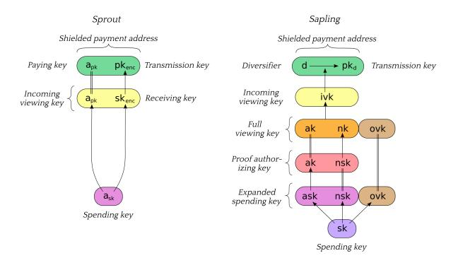
[Sprout] The receiving key  $sk_{enc}$ , incoming viewing key  $ivk = (a_{pk}, sk_{enc})$ , and shielded payment address  $addr_{pk} = (a_{pk}, pk_{enc})$  are derived from the spending key  $a_{sk}$ , as described in § 4.2.1 'Sprout Key Components' on p. 31.
