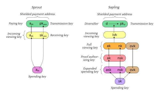
[Sprout] The receiving key  $sk_{enc}$ , incoming viewing key  $ivk = (a_{pk}, sk_{enc})$ , and shielded payment address  $addr_{pk} = (a_{pk}, pk_{enc})$  are derived from the spending key  $a_{sk}$ , as described in §4.2.1 'Sprout Key Components' on p. 30.
