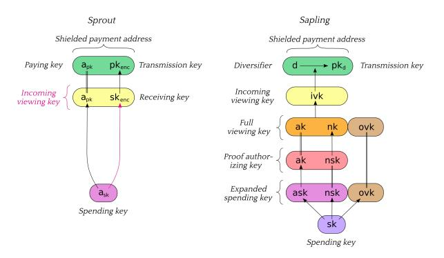
[Sprout] The receiving key  $sk_{enc}$ , incoming viewing key  $ivk = (a_{pk}, sk_{enc})$ , and shielded payment address  $addr_{pk} = (a_{pk}, pk_{enc})$  are derived from the spending key  $a_{sk}$ , as described in § 4.2.1 'Sprout Key Components' on p. 29.
